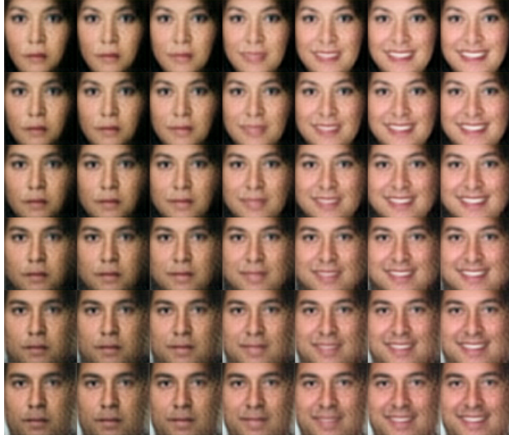
Figure 4.5: Examples of generated images when the gender and joy labels are modified. Left to right shows increased joy evidence and top to bottom shows increased male gender probability.
