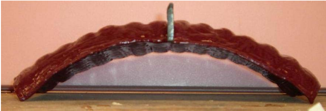
Figure D - 6 : Partial Deflection Back
