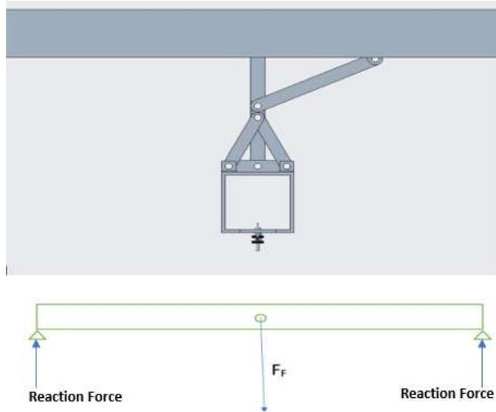
*Figure 7 Loads and Stresses on Pendulum Support Beam*
