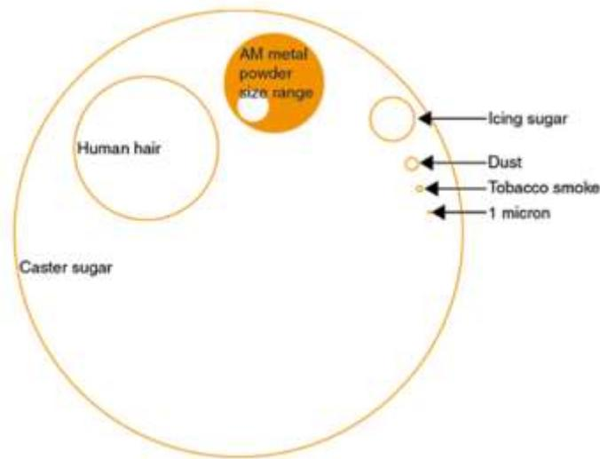
*Figure 54 Particle Size Comparison Image Credit: (Reinshaw)*
