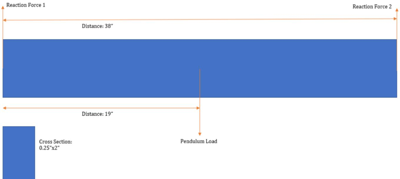
*Figure 23 Pendulum Support Beam Static Free Body Diagram*
