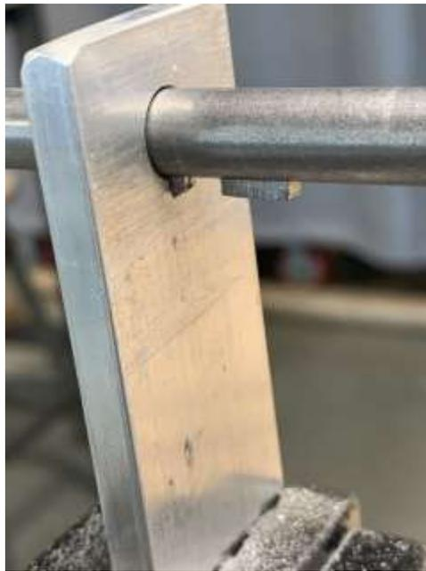
*Figure 39 Crank Arms With Keyway A*
