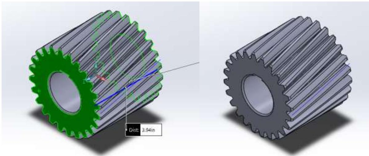
*Figure 53 Helical Gear*
