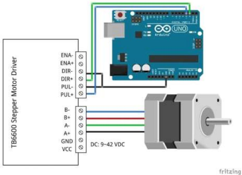
*Figure 44 Arduino – Motor Configuration*
