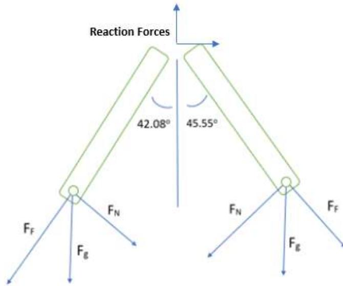
*Figure 8 Loads and Stresses on the Pendulum*
