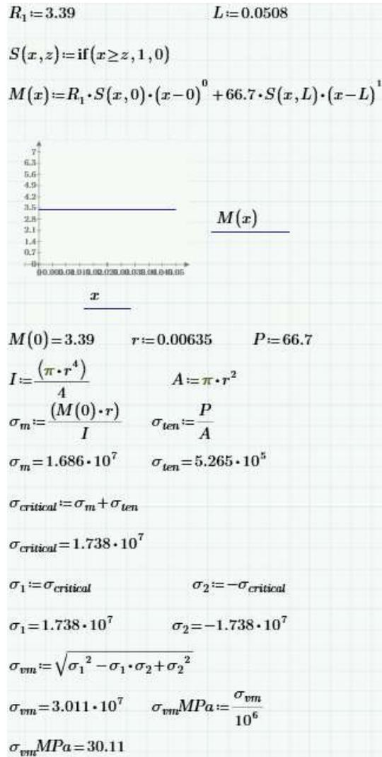
*Figure 27 Build Plate Shaft Stress Analysis*
