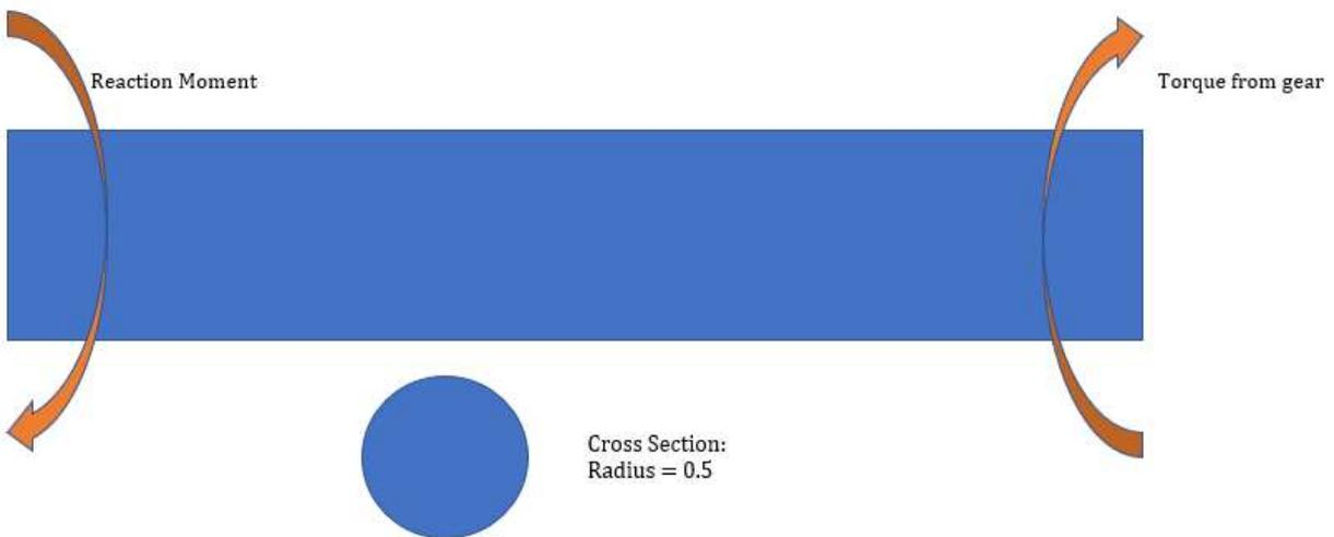
*Figure 17 Crank Shaft Static Free Body Diagram*
