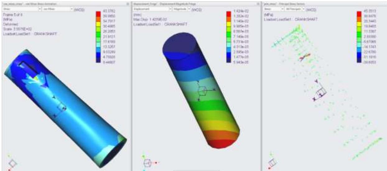
*Figure 16 Crank Shaft FEA*
