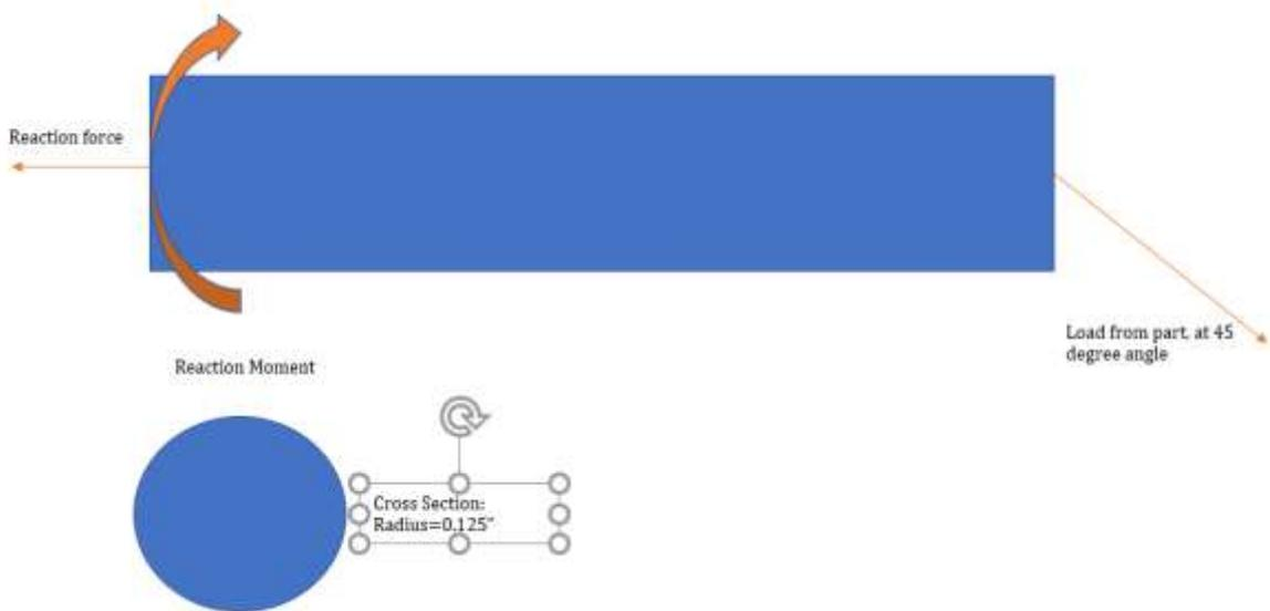
*Figure 26 Build Plate Shaft Static Free Body Diagram*
