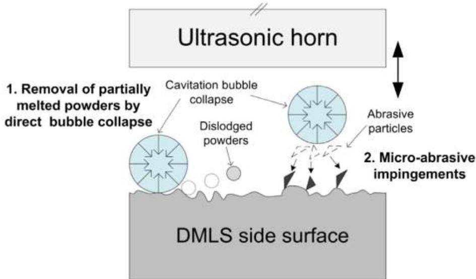
*Figure 2: Ultrasonic Cleaning with Liquid Medium Tan, K., & Yeo, S. (2017)*
