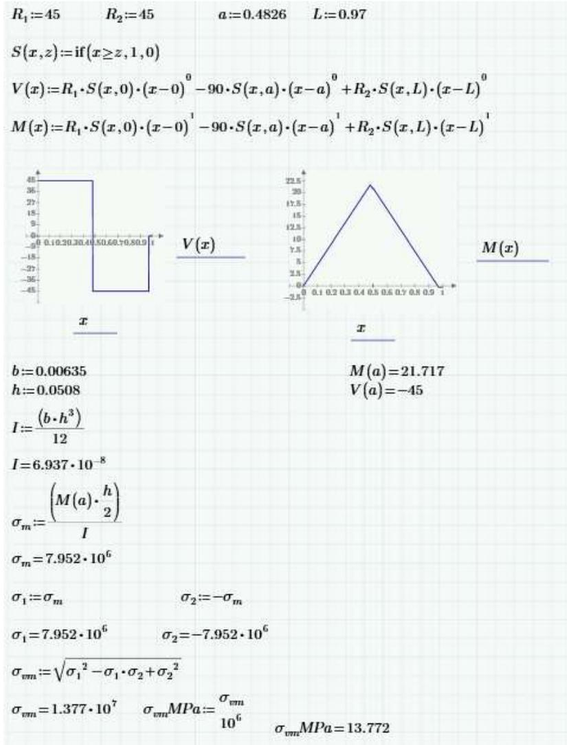
*Figure 24 Pendulum Support Beam Stress Analysis*
