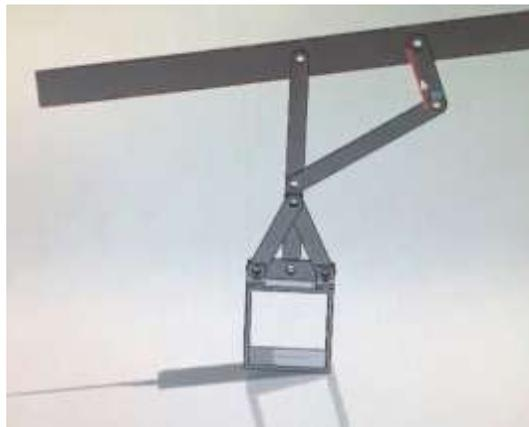
*Figure 5 Four-bar Linkage*
