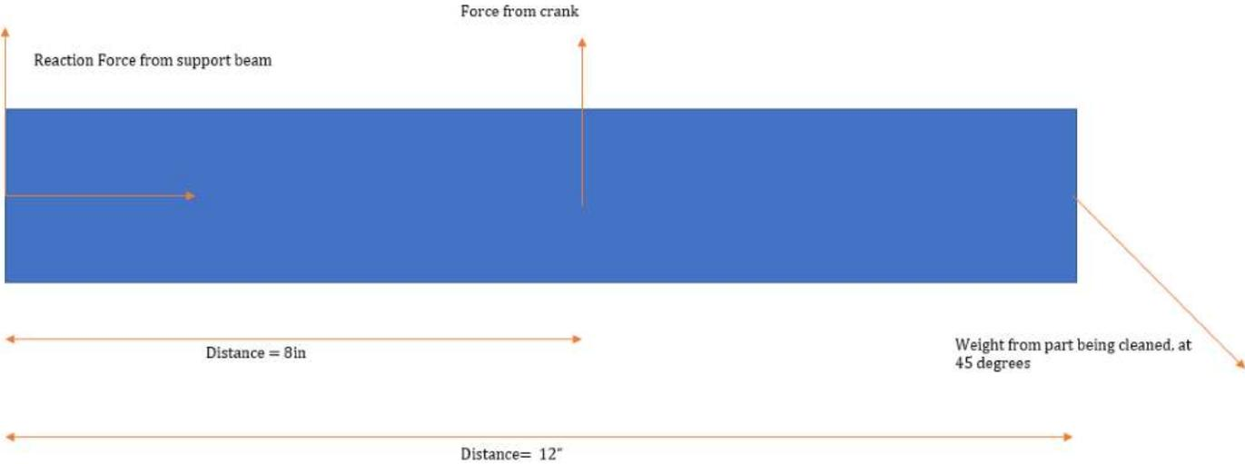
*Figure 20 Pendulum Link Static Free Body Diagram*
