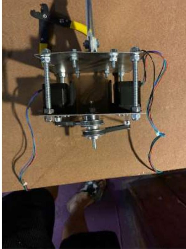
*Figure 36 Motor Mount with the Motors*
