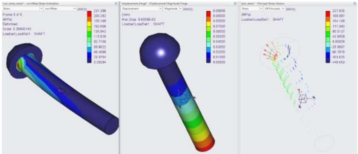
*Figure 25 Build Plate Shaft FEA*
