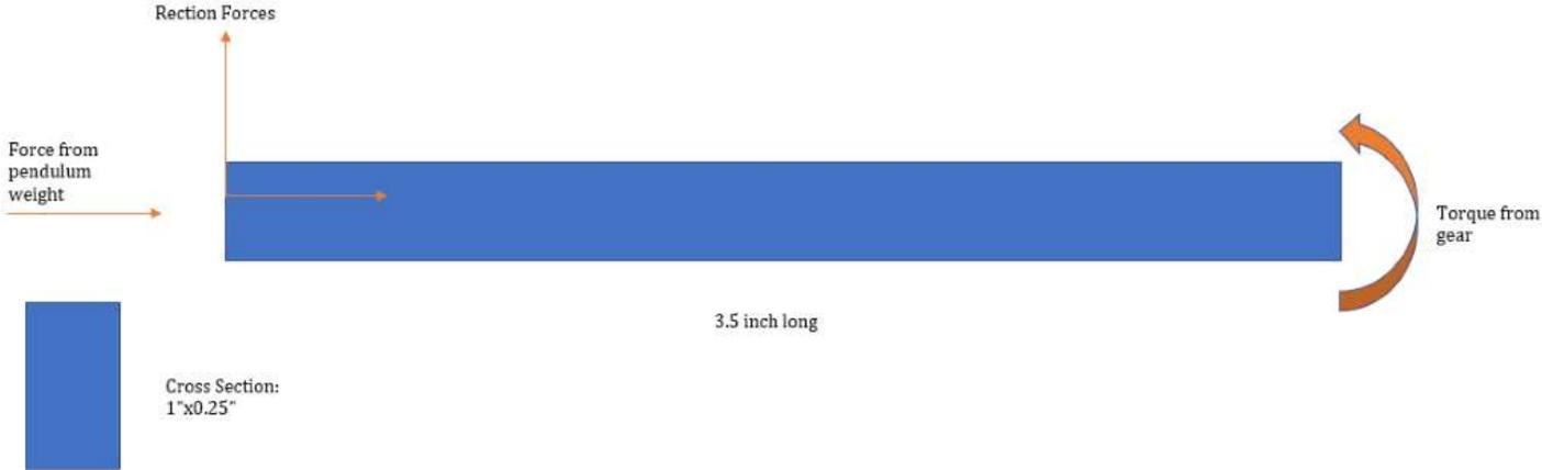
*Figure 14 Crank Static Free Body Diagram*
