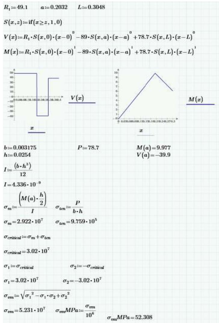
*Figure 21 Pendulum Link Stress Analysis*
