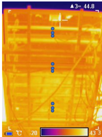
Figure 36: Data Collection Points for the Back of the Novel PV/T System
