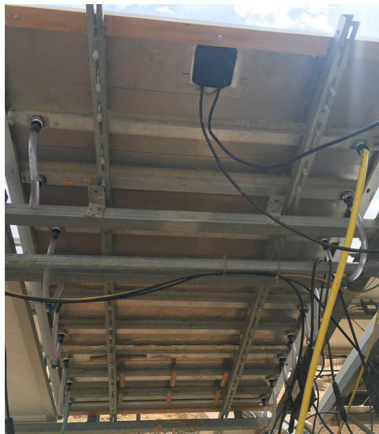
Figure 19: Novel PV/T System
