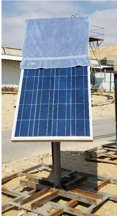
Figure 25: Effect of PV Panel Coverage on Power Output Experiment - Top Half Covering
