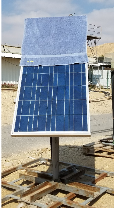
Figure 8: Effect of PV Panel Coverage on Power Output - Top Half Covering
