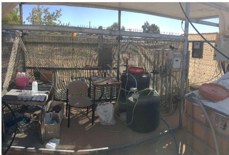
Figure 6: Effect of Temperature on RO Processes Experiment Set Up
