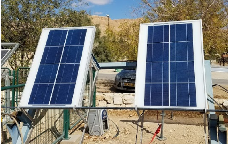
Figure 9: Effect of Localized Cooling and Heating on PV Panel Power Output - Set Up
