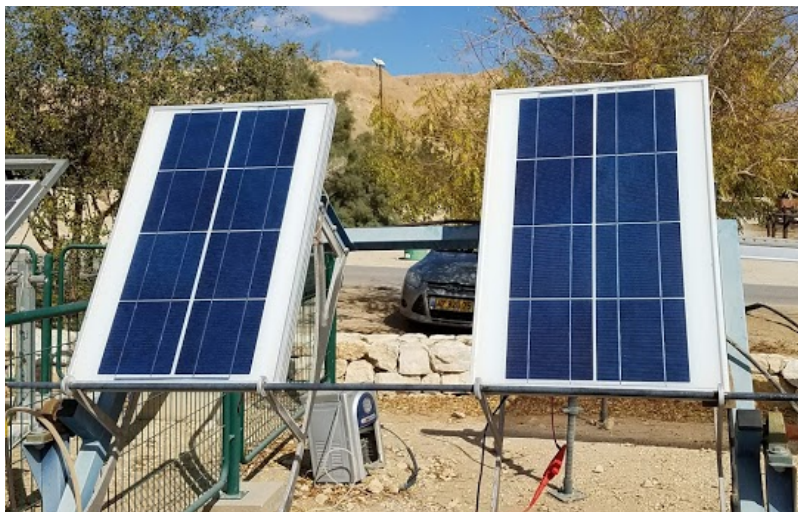
Figure 26: Effect of Localized Cooling and Heating on PV Panel Power Output Experiment - Set Up
