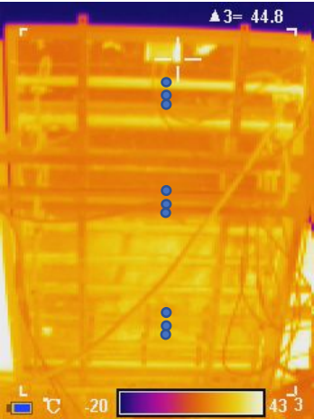
Figure 11: Measurement Points for Back of Novel PV/T System
