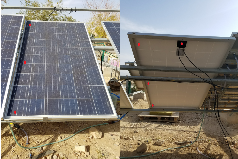
Figure 7: Measurement Points for Baseline PV Temperature and Power Data Collection
