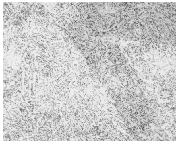
FIGURE 20: 4140 LOW ALLOY STEEL MICROSTRUCTURE: LONGITUDINAL.
