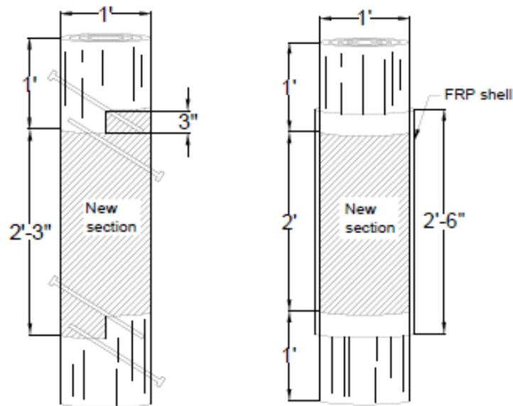
**Figure 10:** Splicing with Bolt Fasteners, on left and Splicing with FRP Wrap, on right (White et al., 2007)
