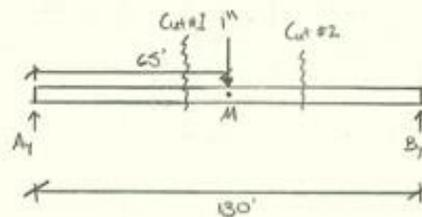
Greatest Moment Will Occur @ Midspan (M). Thus, The Unit Load Was Placed @ Midspan (M).
