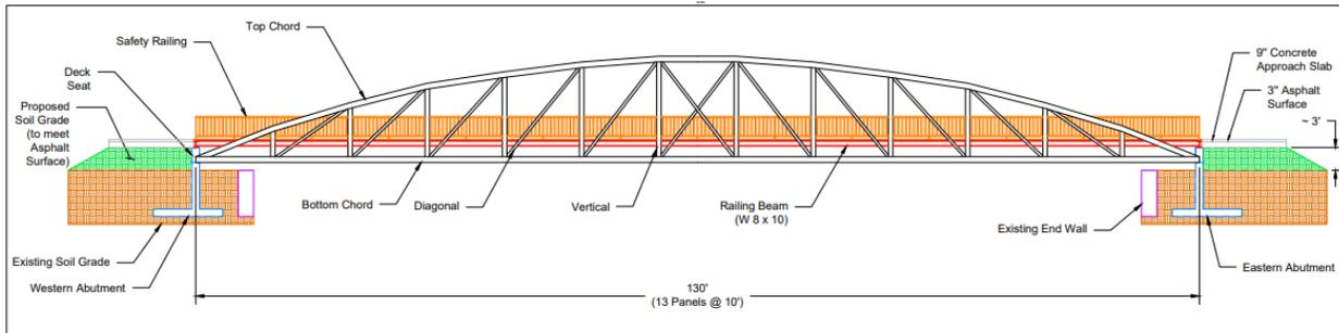
**Figure 15:** Elevation View of Bridge and Abutments
