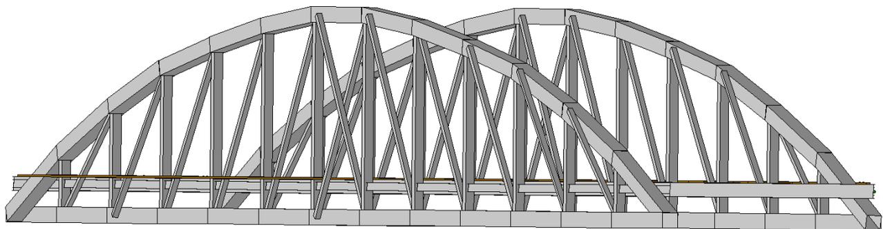
**Figure 14:** Isometric View of the Final Bridge Design
