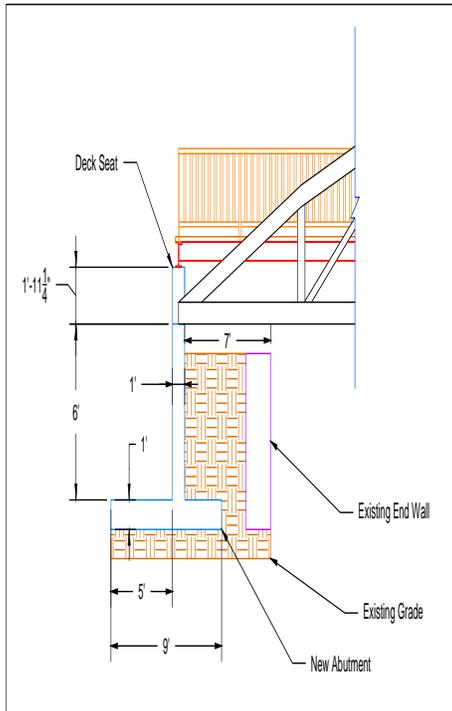
ABUTMENT REINFORCEMENT DETAIL
