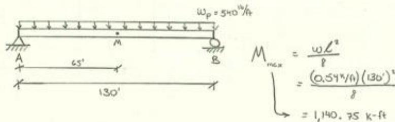
The Pedestrian Loading Generates A Maximum Moment of 1,140.75 ft @ Point M on the beam.
