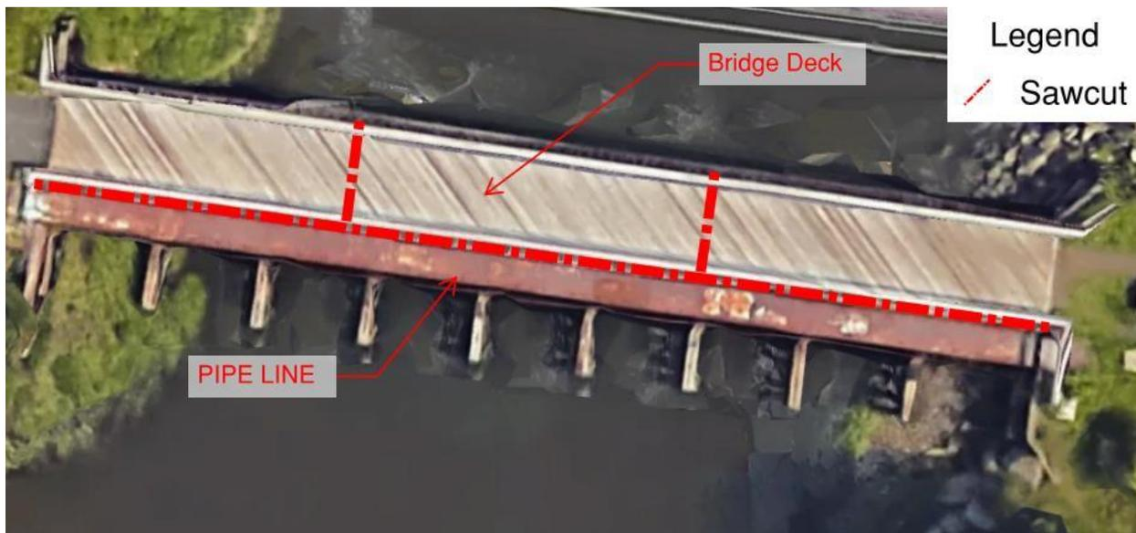
**Figure 18:** Sawcut Plan
