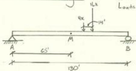
As Per Ped. Spec. - 3.2, The Vehicle Loading 'shall Be Placed To Produce The Maximum Load Effects'.
