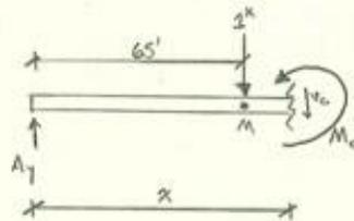
$$\begin{aligned} \sum M_{cut} &= 0 \\ 0 &= A_y(x) - (1^k)(x-65') - M_c \\ M_c &= (0.5^k)x - (1^k)x + 65^k-ft \\ M_c &= 65^k-ft - 0.5^kx \\ (65' \leq x \leq 130') \end{aligned}$$
