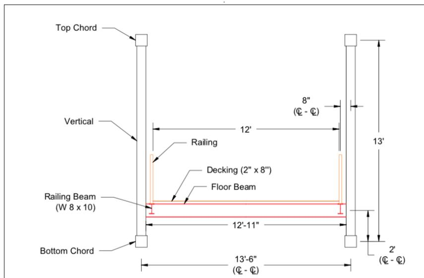
**Figure 16:** Cross Section View of Bridge
