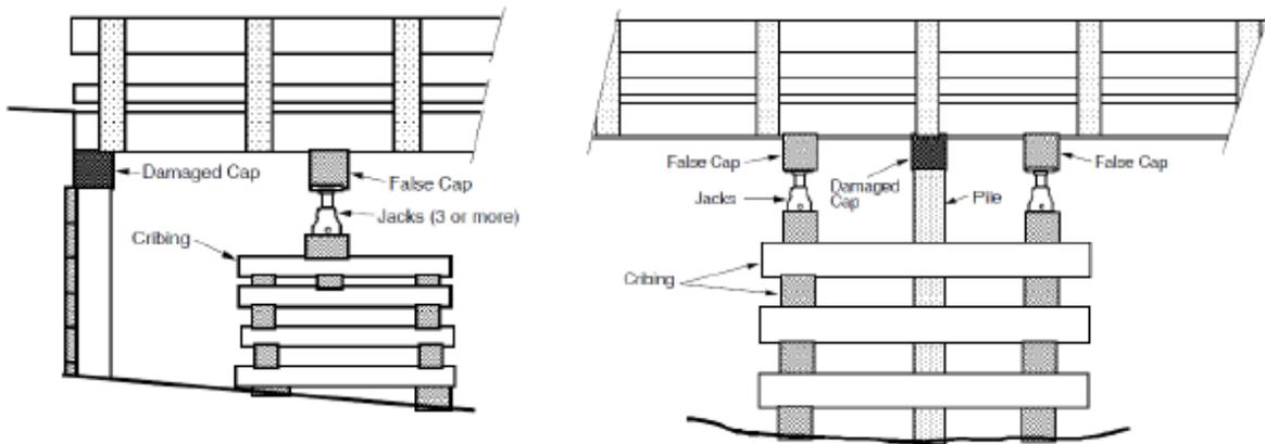
**Figure 11:** Pile Cap Jacking and Rehabilitation (Johnson, 2002)
