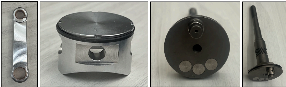
Figure 9: Piston rod (top left), piston head (top right), and crankshaft (bottom).
