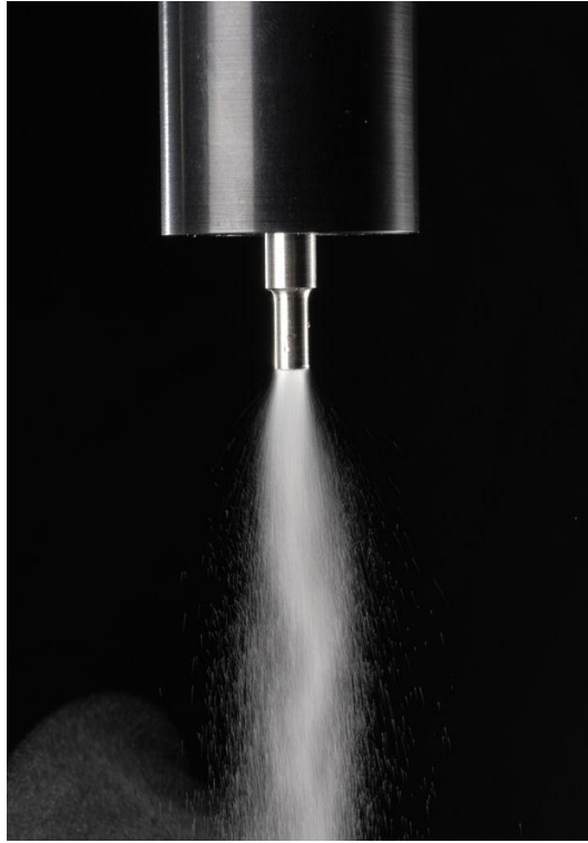
Figure 21: This is an example of the fine spray emitted by the atomizing nozzles.
