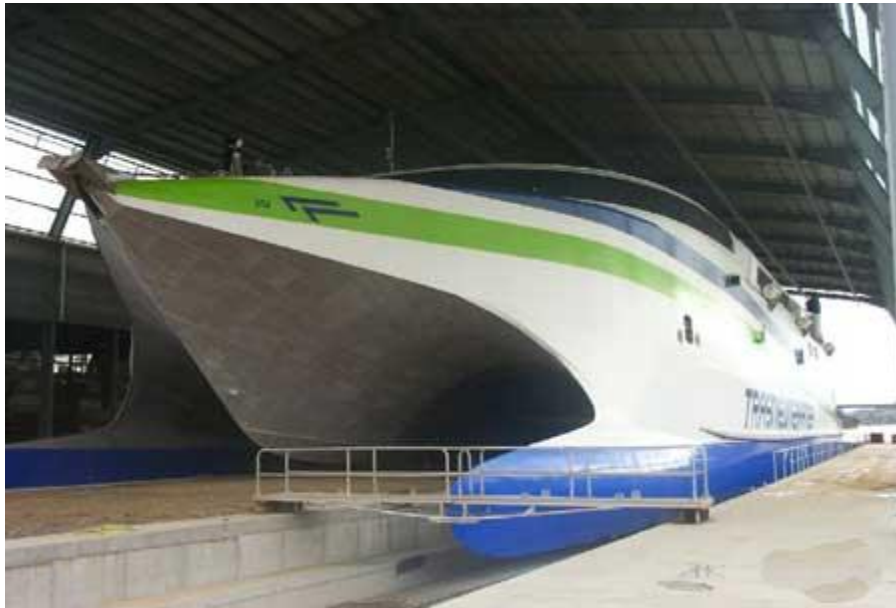
Figure 15: This close-up view of the hull shows how the wave-piercing design works.
