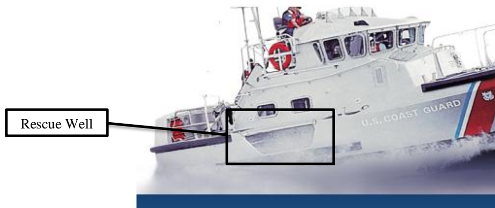
Figure 33: A close up of the vessel's "Rescue Well".
