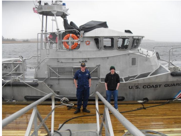
Figure 37: The 47-foot Motor Lifeboat has very limited options due to its small size. (Also to be noted, you can easily see the sharp angles that one would need to overcome in order to move a patient to the inner chamber if the ship.)
