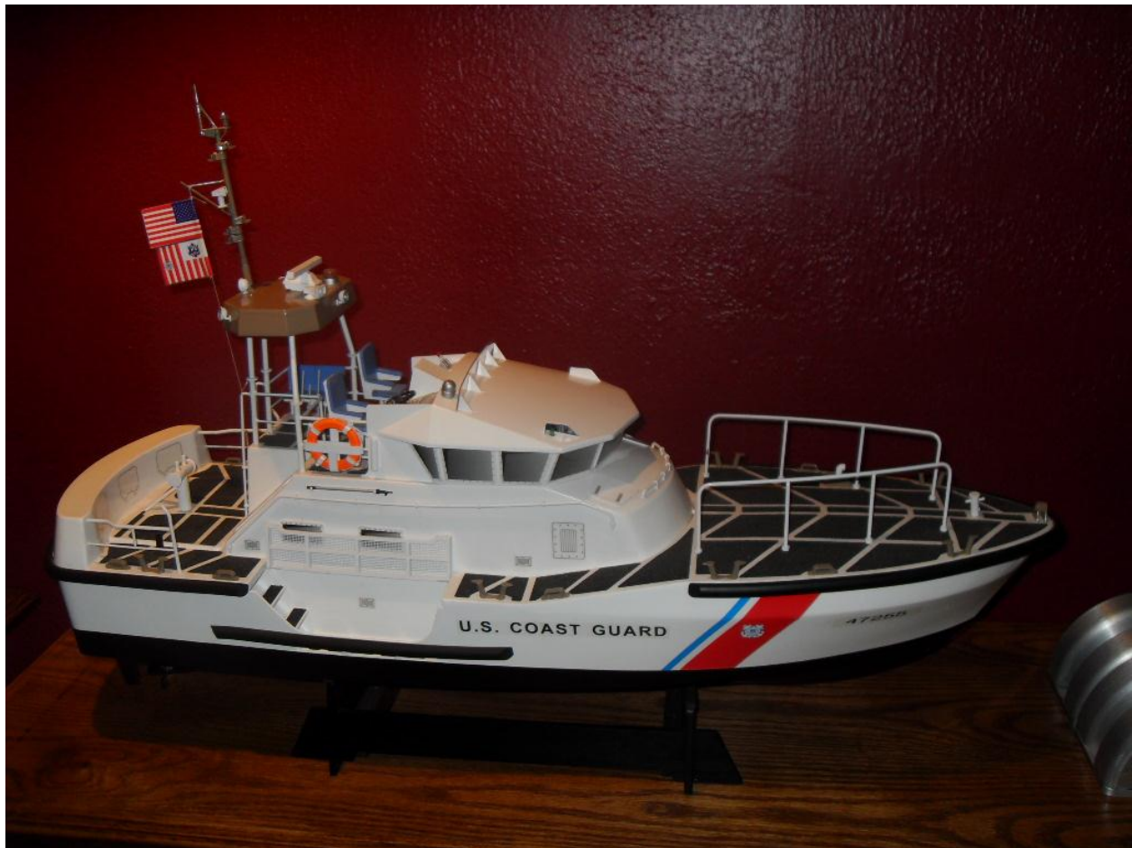
Figure 35: The closed bridge of the ship provides full protection, while the open bridge provides a 360 degree view.
