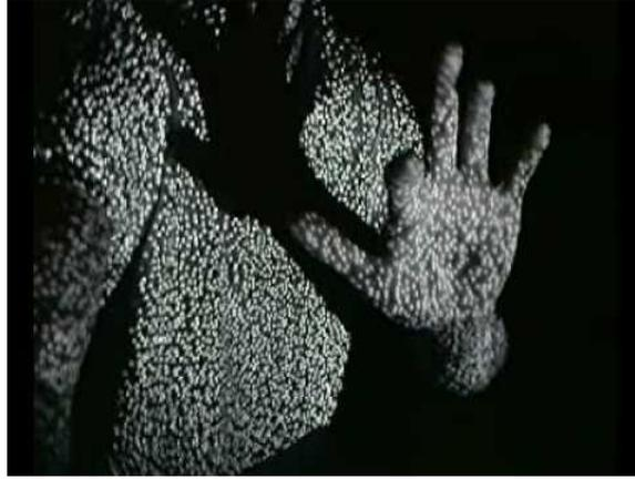
*Figure 10. IR dot pattern projected onto a scene of a body and hand*
