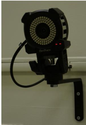
*Figure 3. Motion Capture camera used as one of many in a typical motion capture system.*
