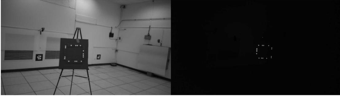
Figure 25. Raw luminance image with no IR filter on the left, and raw luminance with an 850nm IR filter on the right
