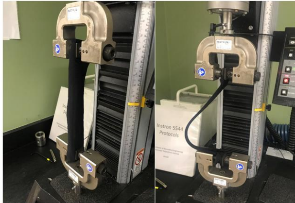
Figure 13: Before and After Failure testing of the Sock Material
