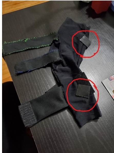
Figure 16: Photo of the Dislodged Velcro Pieces After Washing
