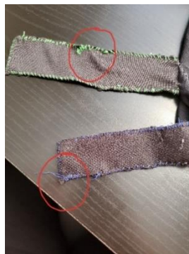
Figure 17: Photo of the Frayed Thread After Washing
