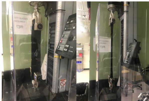
Figure 14: Progression of extension for Strap Material during Failure Testing
