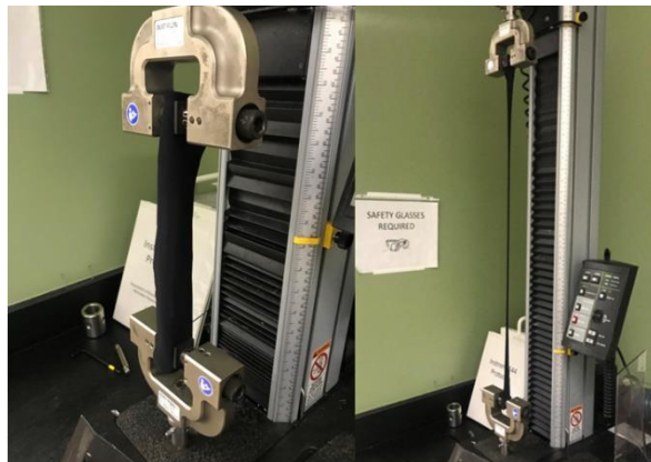
Figure 15: Progression of Extension for Sock Material during Failure Testing
