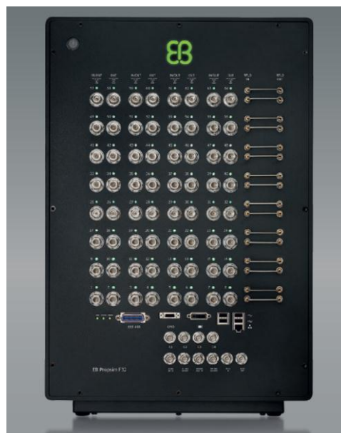
Figure 11: Elektrobit Prosim F32, radio channel emulator [24]. The F32 model has the capacity to support as many as 32 distinct RF channels with 16 bidirectional nodes. This channel emulator can also emulate fading.
