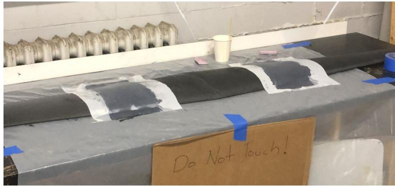
**Figure 61: Wing Assembly Lay-up**
