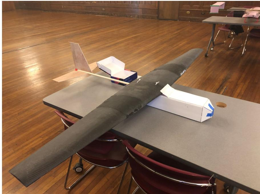
**Figure 85: Isometric View of Glide Test Model**
