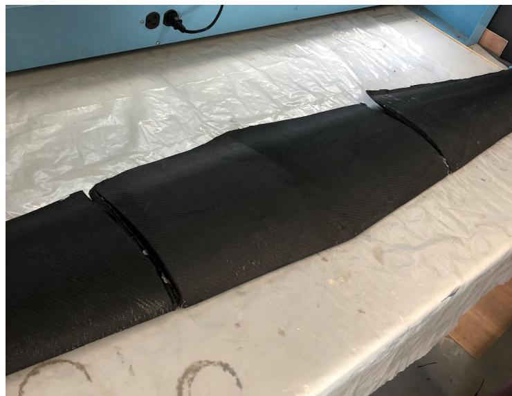
**Figure 60: Wing in Three Sections**
