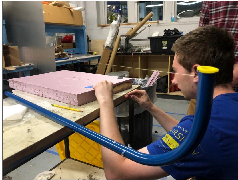
**Figure 56: Application of Splines for Foam Cutting**
