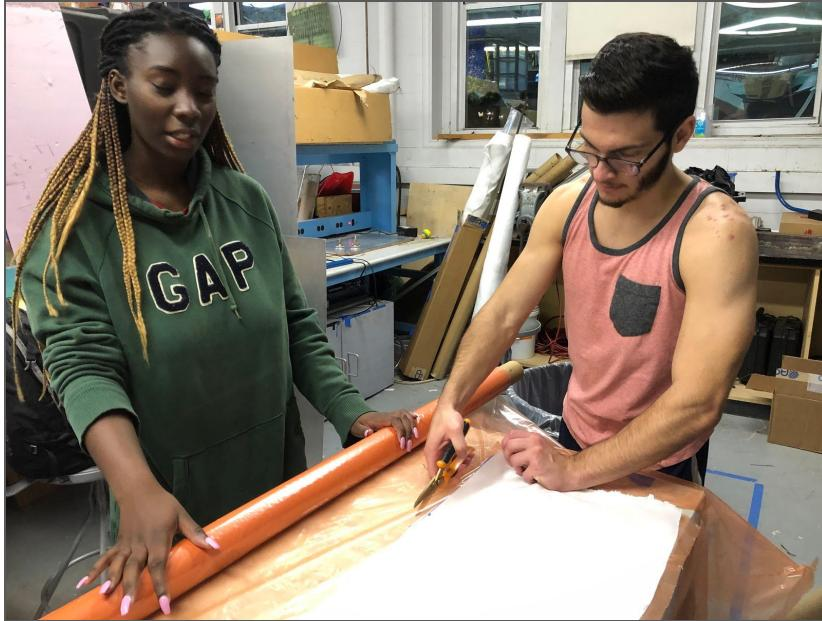
**Figure 58: Cutting Breather and Wadding**
