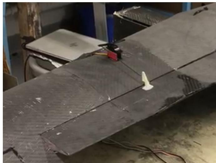
**Figure 45: Push-Pull Linkage System**
