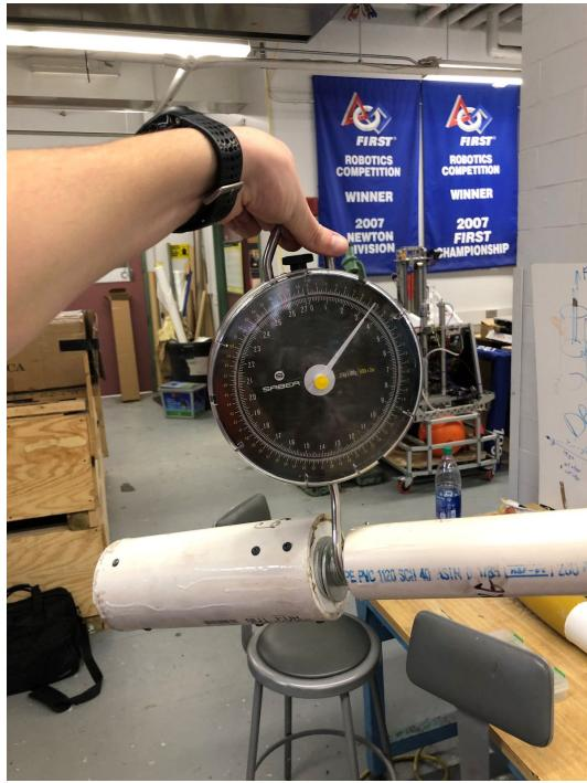
**Figure 83: Weight for Wing Load Test**
