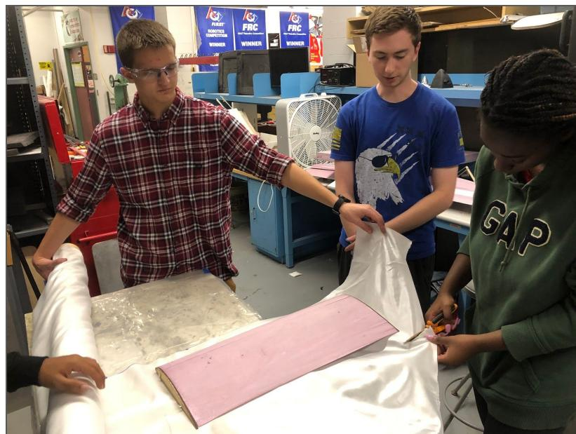
**Figure 57: Cutting Peel-Ply**
