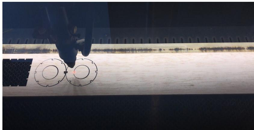
**Figure 32: Process of Laser Cutting Circular Fuselage**
