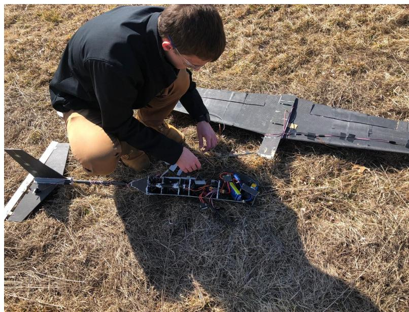
**Figure 88: Flight Test Wreckage**
