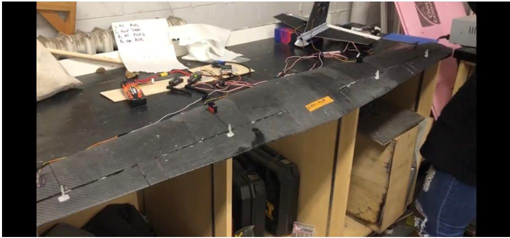
**Figure 63: Ailerons and flaps control surfaces**
