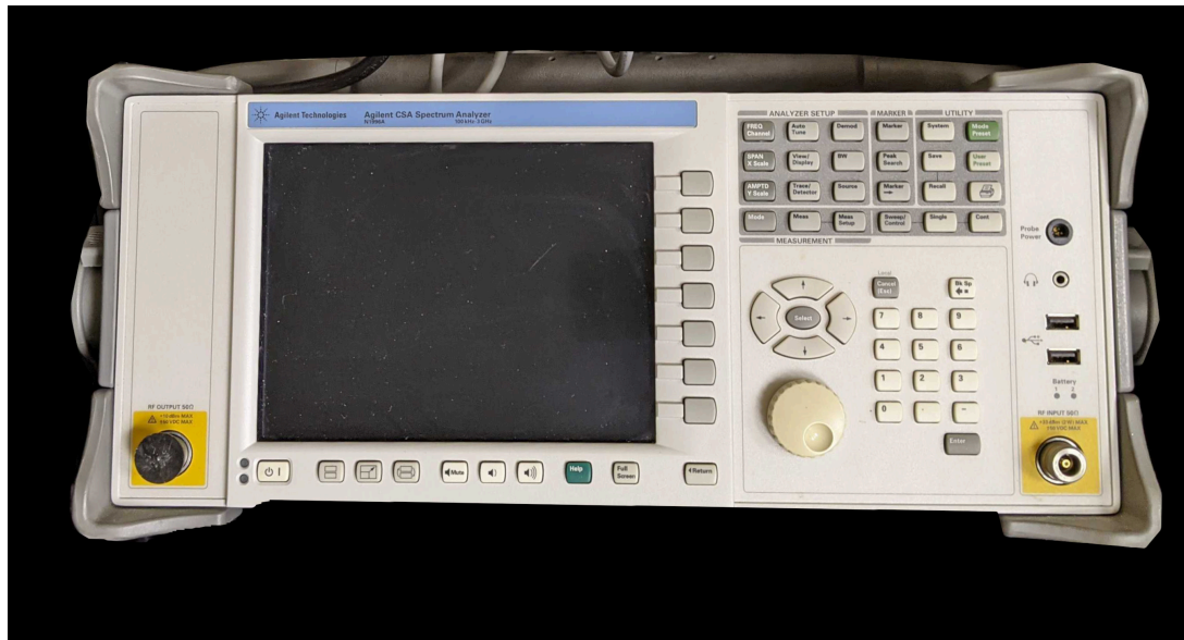
Figure 4.7: A picture of the Agilent CSA Spectrum Analyzer N1996A. It operates from 100 kHz to 3 GHz.
