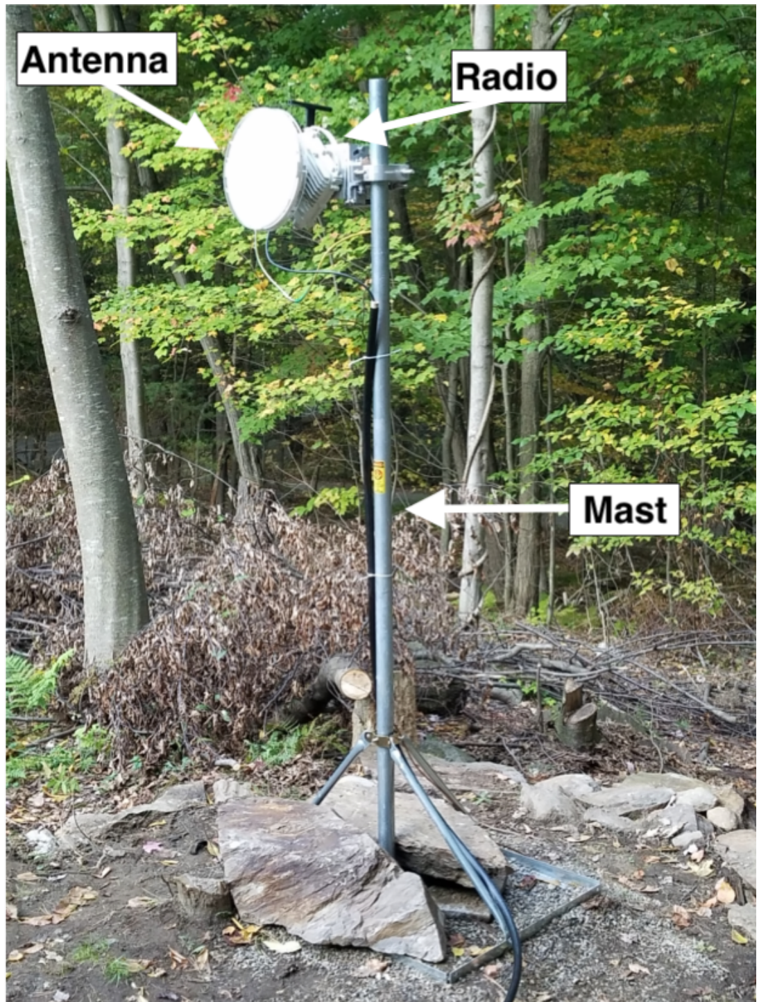
Figure 3.1: Four of these commercial radios were used to create two separate communication links, as it would create extra work to turn the middle radio and have to realign the radios each time. This configuration also allows a seamless data transmission through the two data links.
