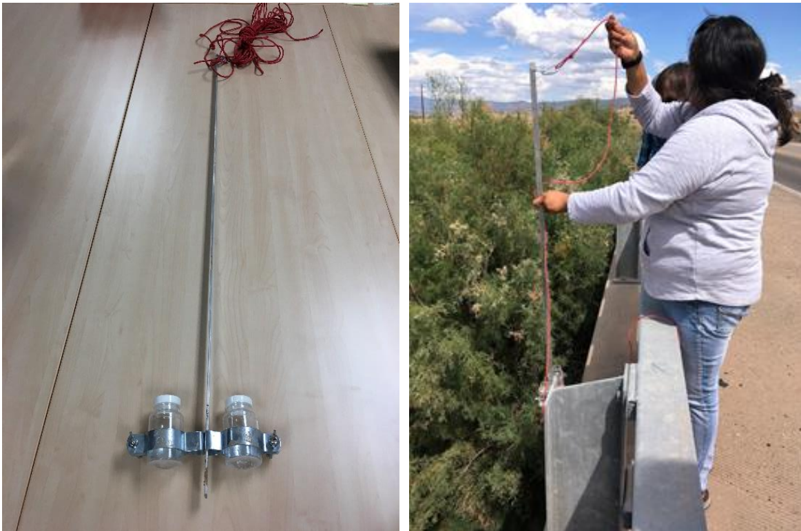
Figure 4.1: Water sampling device (left). Device being lowered off of San Ysidro bridge (right).
