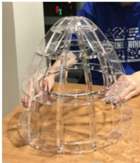
Figure 5-19: The Assembled Nacelle Frame
