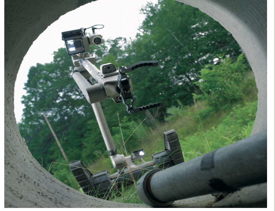
A PackBot prepares to grasp a suspicious object
