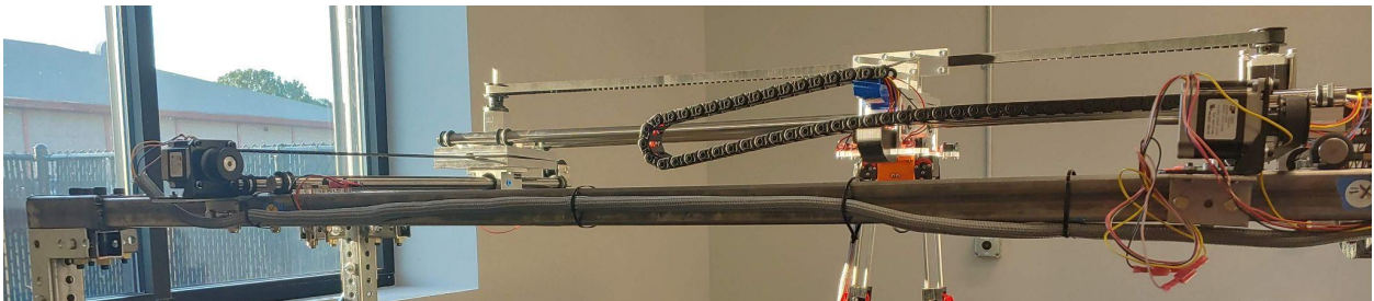
Figure 5.2: Wire Harness Across the Robot Frame
