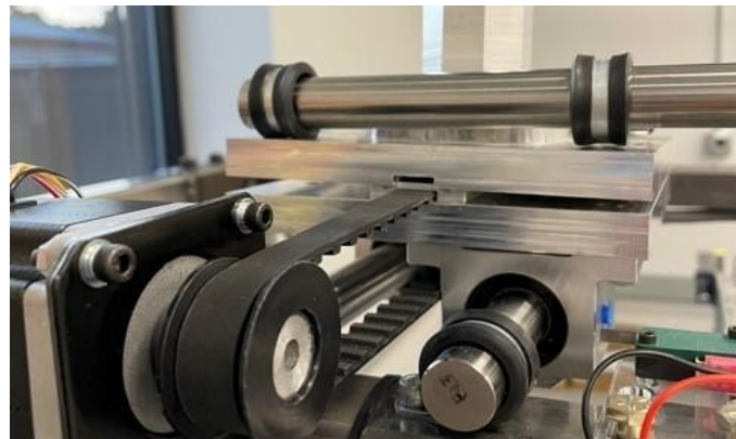
Figure 3.1: Robot Coordinate Frame Figure 3.2: Upper cart sitting unevenly on the lower cart The following solutions were identified to help improve movement of the robot:
