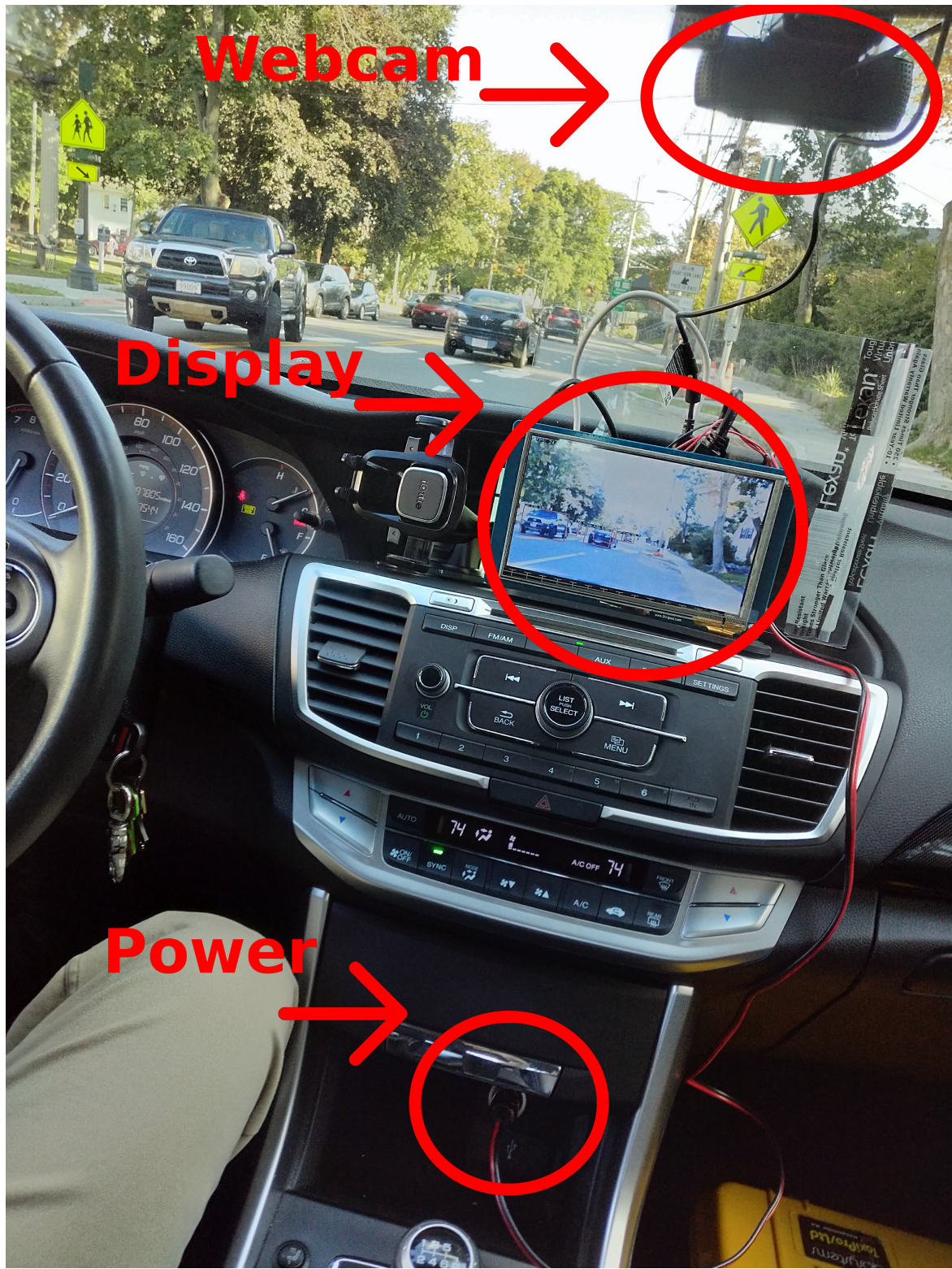
Figure 3.7: Circled in red above are each of the connections needed for system operation. From top to bottom the items shown include the webcam, assembled system, and the power connector.
