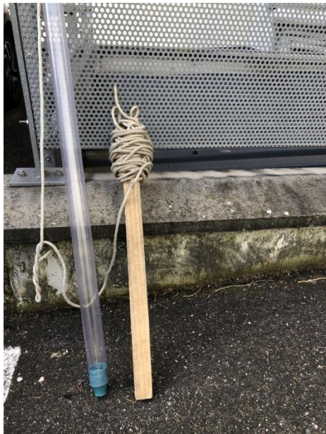
Figure 9: Bailer used to collect samples from bridges
