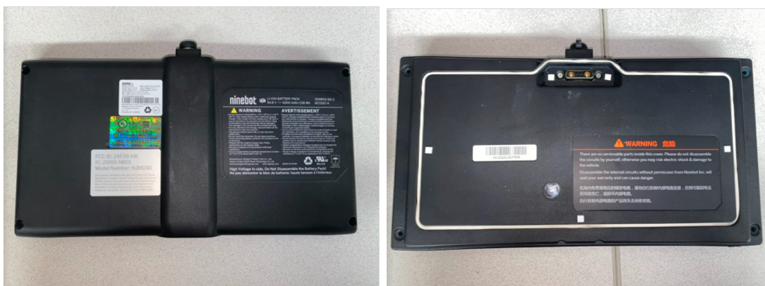
Figure 3.5: Lithium-ion Battery removed from Ninebot S Chassis.
