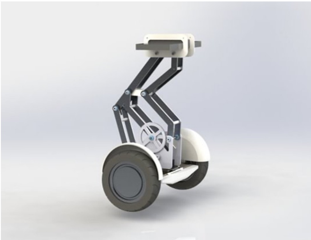
Figure 3.11: Prototype version of the Ninebot S with attached jumping mechanism.
