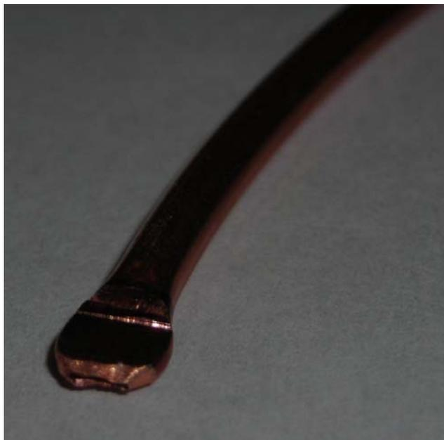
**Figure 5-5: Flattened end of the copper tubing**
