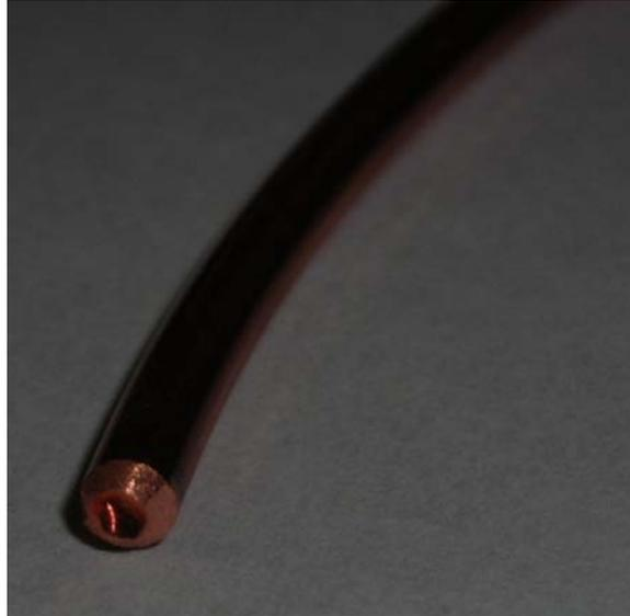
**Figure 5-3: End of tubing after cut and sanded**
