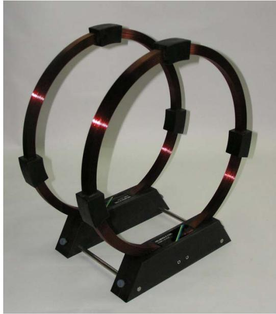
**Figure 3-1: Helmholtz Coil Example Construction**
