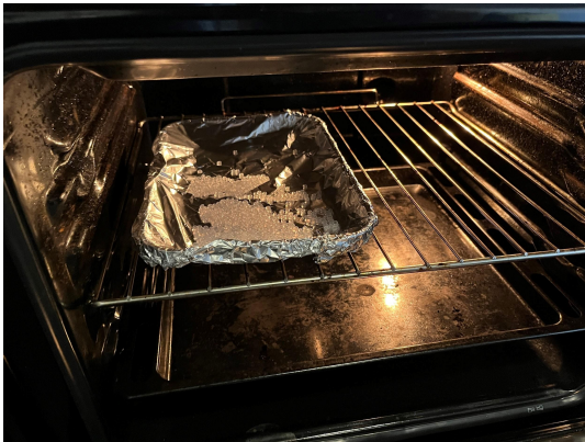
Figure B2: Polypropylene cooking in the oven
