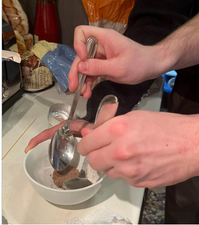
Figure B3: Mixing PP and broken down nut shells
