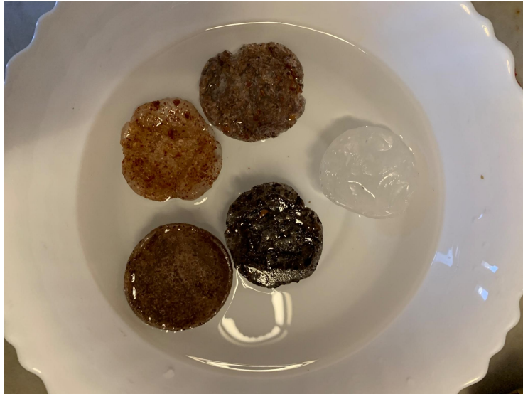
Figure B7: WPCs soaking in a bowl of water
