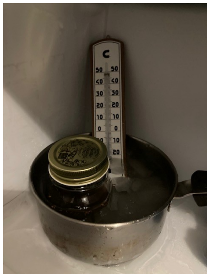
Figure A1: Setup of cellulose extraction using an ice bath at -6C to cool NaOH solution containing crushed argan nuts.
