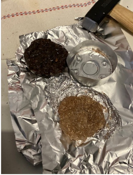
Figure B5: WPC after forming to candle mold shape
