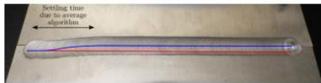
Figure 5. FANUC Weldment: Corrected Path (Blue); Real Path (Red)
