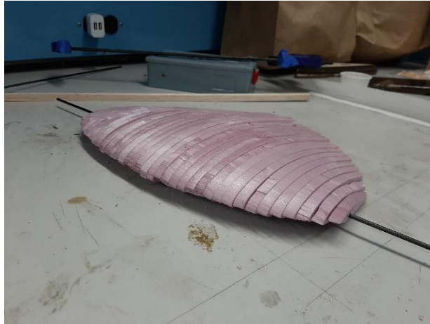
Figure 48. Final Wing Before Sanding.
