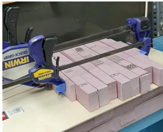
Figure 45. Glue Curing Setup
