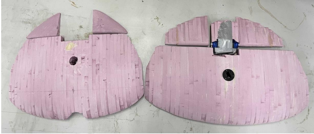
Figure 41. Wing and Wing with 27.5% Increased Wingspan
