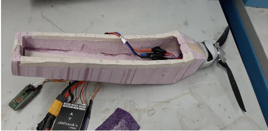
Figure 40. Final Fuselage Iteration
