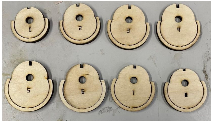
Figure 50. Fuselage Balsa Guides
