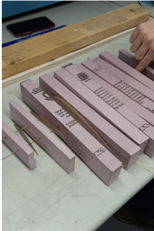
Figure 44. Aligning Spars and Foam
