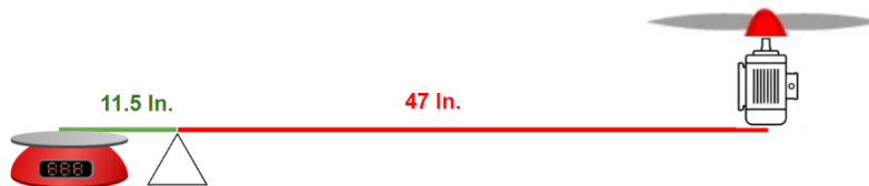
Figure 36. Static Thrust Testing Diagram
