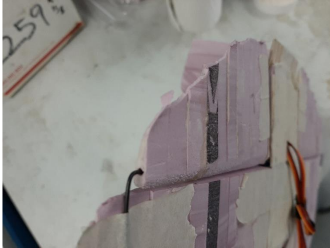
Figure 42. Control Rods Inserted in Elevon
