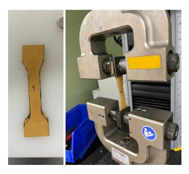
Figure 5.5: Samples of Leather Used for Mechanical Testing.
