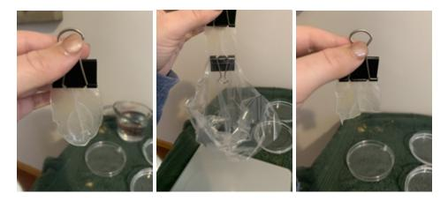
Figure 4.9: At Home Mechanical Testing of Decellularized Spinach Leaves. The image on the left is the decellularized spinach leaf prior to the mechanical test. The middle image shows the mechanical test being performed. The image on the right shows the torn leaf from mechanical
