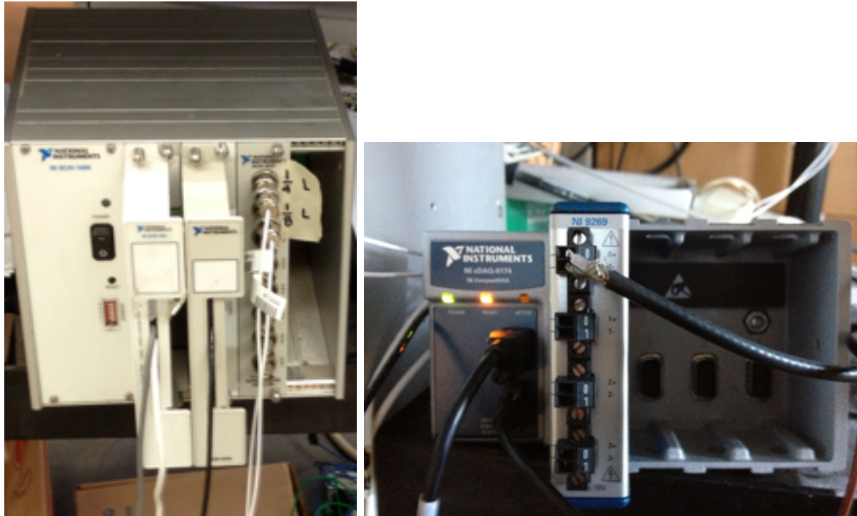
Figure 4 NI SCXI-1000 wired into the sensors used for this setup and the lab computer (Left) and NI-9269 for outputting voltage plugged into the NI cDAQ-9174 Chassis (Right).
