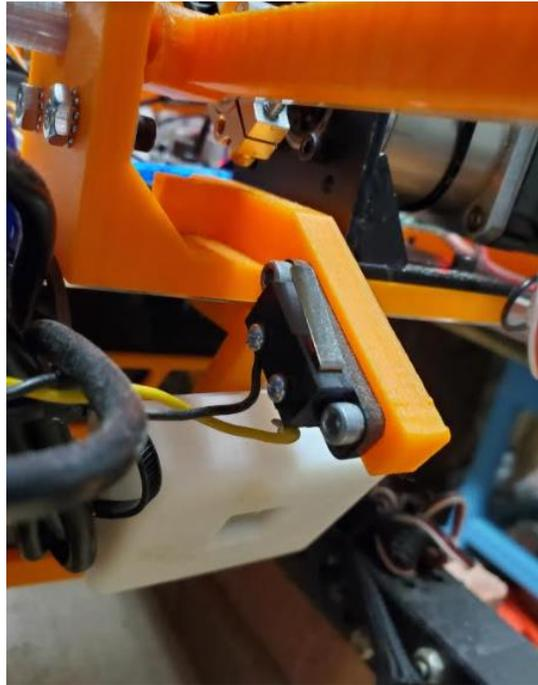
**Figure 39: Picture of Limit Switch Mounted Below Shoulder Link of Arm**
