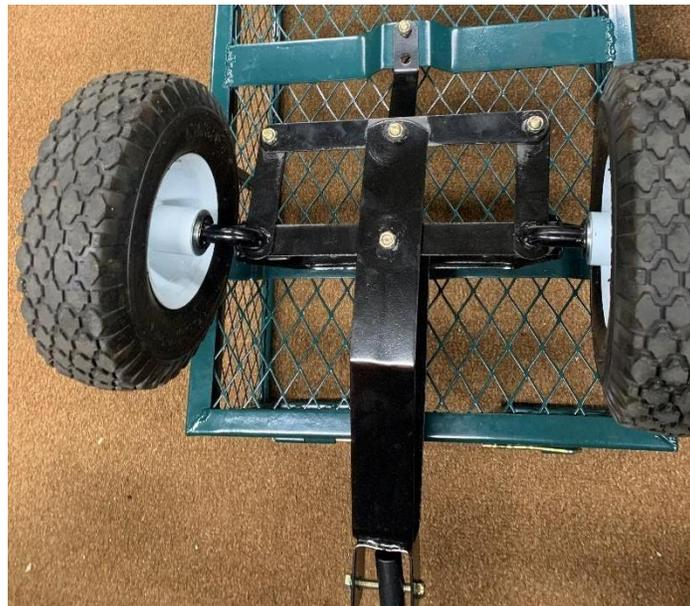
**Figure 64: Current Basebot Steering Mechanism View 1**
