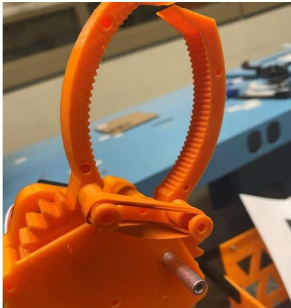
*Figure 12: Rubber Bands Attached to the Gripper*
