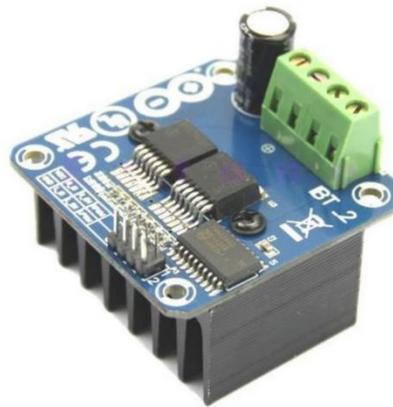
**Figure 88: H-Bridge Motor Driver Selection**
