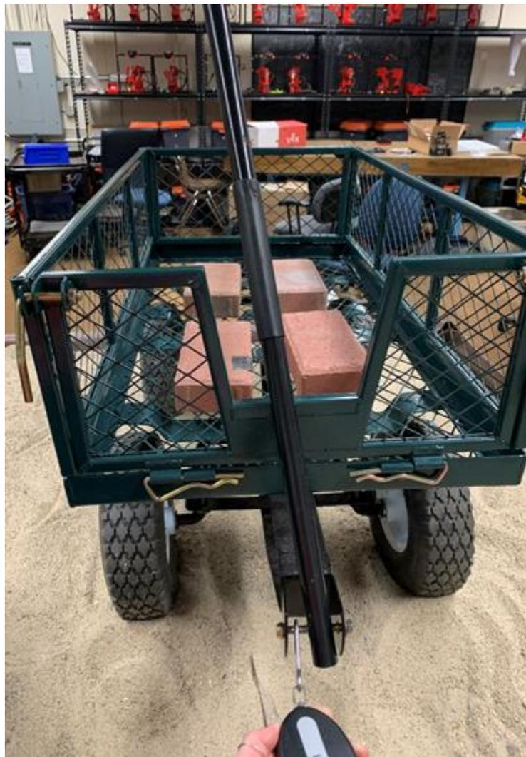
**Figure 90: Coefficient of Friction of Sand Testing**
