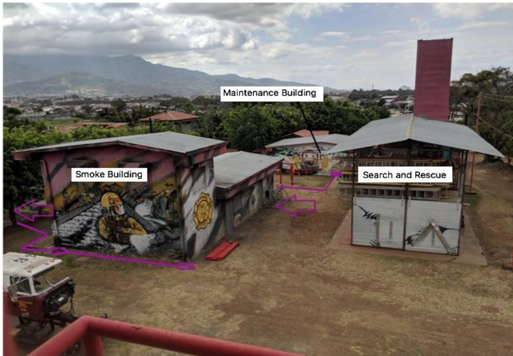
Figure 15: Current piping infrastructure for Smoke Building, Maintenance Building, and Search and Rescue Building. The purple shows that the water flow is currently in the opposite direction of the central training grounds.
