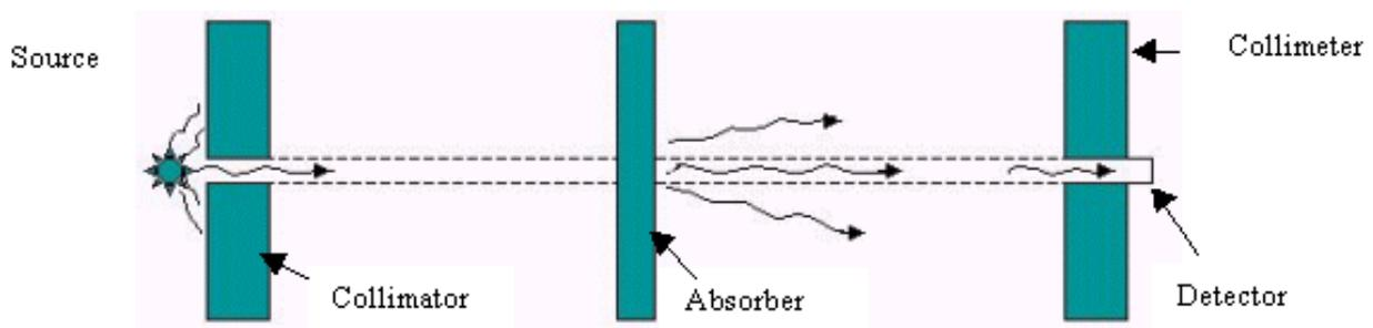
Figure 3 – Narrow beam geometry the simulations and calculations were based on<sup>[F3]</sup>.
