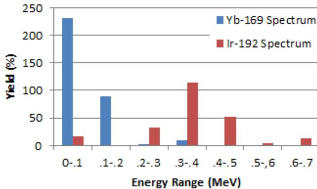
Figure 5 – The spectra of Yb-169 and Ir-192
