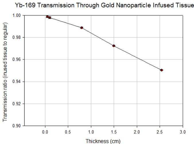
Figure 9 – Yb-169 transmission through gold nanoparticle infused tissue
