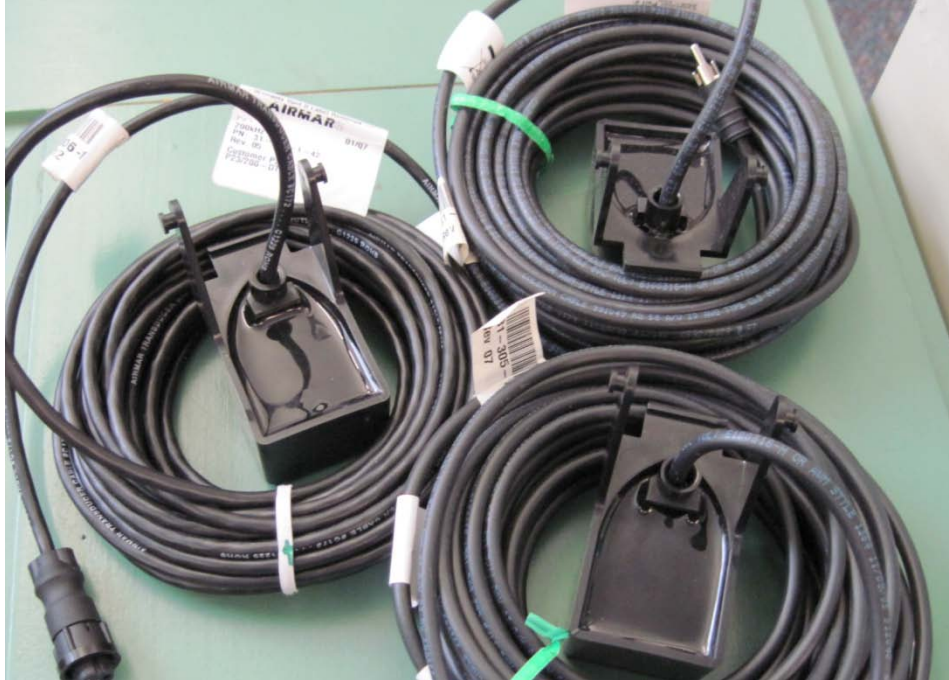
Figure 3: Airmar P23 ultrasonic transducers purchased for the sonar module.
