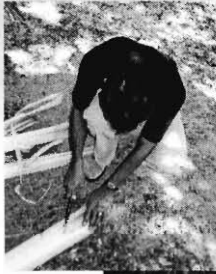
The fibres are extracted, mostly by hand, from the pseudostems of the banana plant
