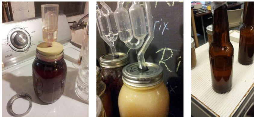
Figure 6: Three design iterations for the micro fermentation experimental setup.
