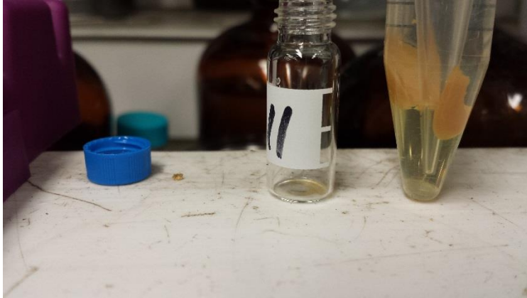
Figure 8: Pipet tip immersed in the dichloromethane extract at the bottom of the centrifuge tube. To the left is a GC sample vial and lid. Notice the solids collected at the phase interface
