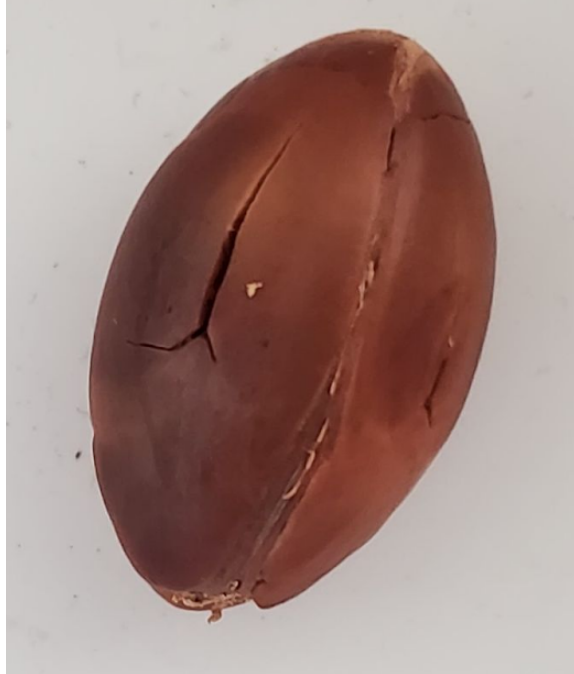
Fig. 11. A photograph illustrating the cracks in the argan nut shell induced by pressure cooking soaked nuts. All nuts that were subjected to this trial were covered in cracks similar to this.
