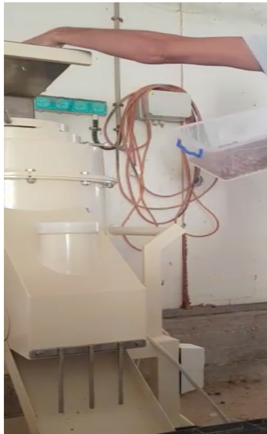
Fig 2. A still from a video by Nadav Solowey showing the current argan nut cracking machine in use at Kibbutz Ketura.
