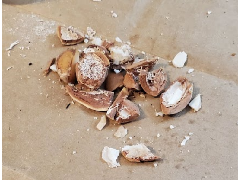
Fig. 6. A crushed argan nut shell and kernel as a result of no force control with the squeezing device.
