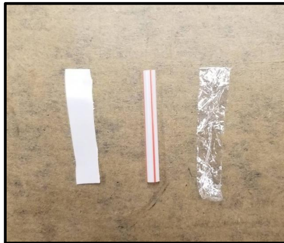
Figure 2: Plastic fibers, from left to right, high-density polyethylene, polypropylene, linear low-density polyethylene.
