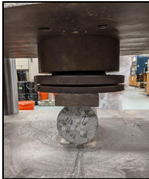
Figure 3: Splitting tensile strength testing apparatus.
