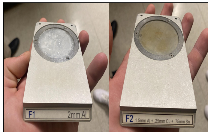
Figure 7: X-ray filters from Massachusetts General Hospital. Image on left is 2mm Aluminum and image on right is 1.5mm Aluminum + .25mm Copper, and .75 mm Tin.
