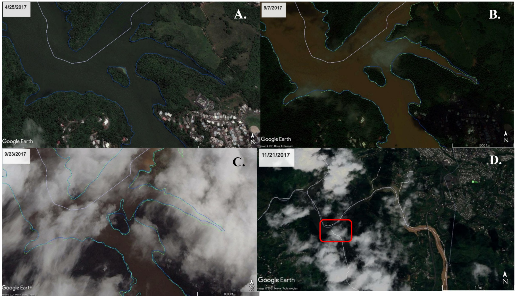
Figure 17(A-D). Sedimentation Before and After Hurricanes Irma and Maria.
