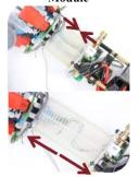
Yoshimura Origami Body: Continuously deformable cable-driven bellows
