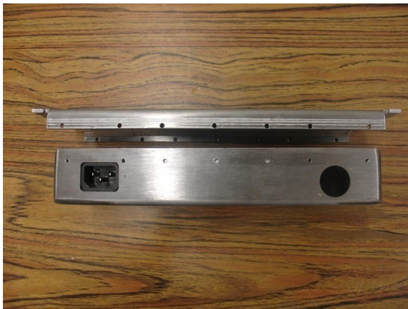
Figure 17: Steel Enclosure Side view, with cutouts for the AC and DC connectors
