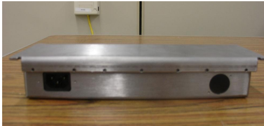
Figure 19: Closed Enclosure Side View. DC and AC connector holes can be seen, as well as screw holes for the lid.
