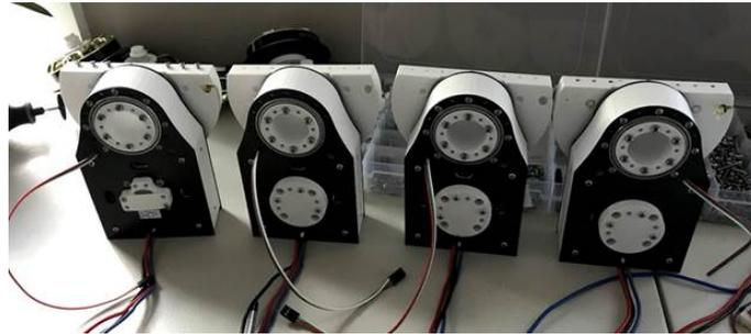
**Figure 38:** *First Capstan Prototypes*
