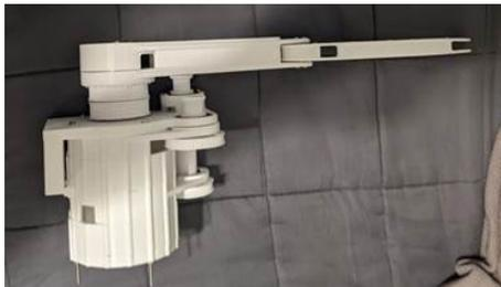
**Figure 12:** *Leg Version 2 without electronics or belts*
