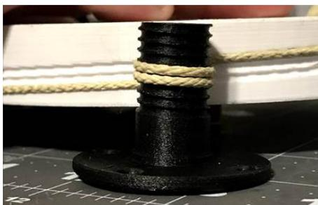
**Figure 26:** *Prototype 1 of Swol Kat Capstan Shoulder*
