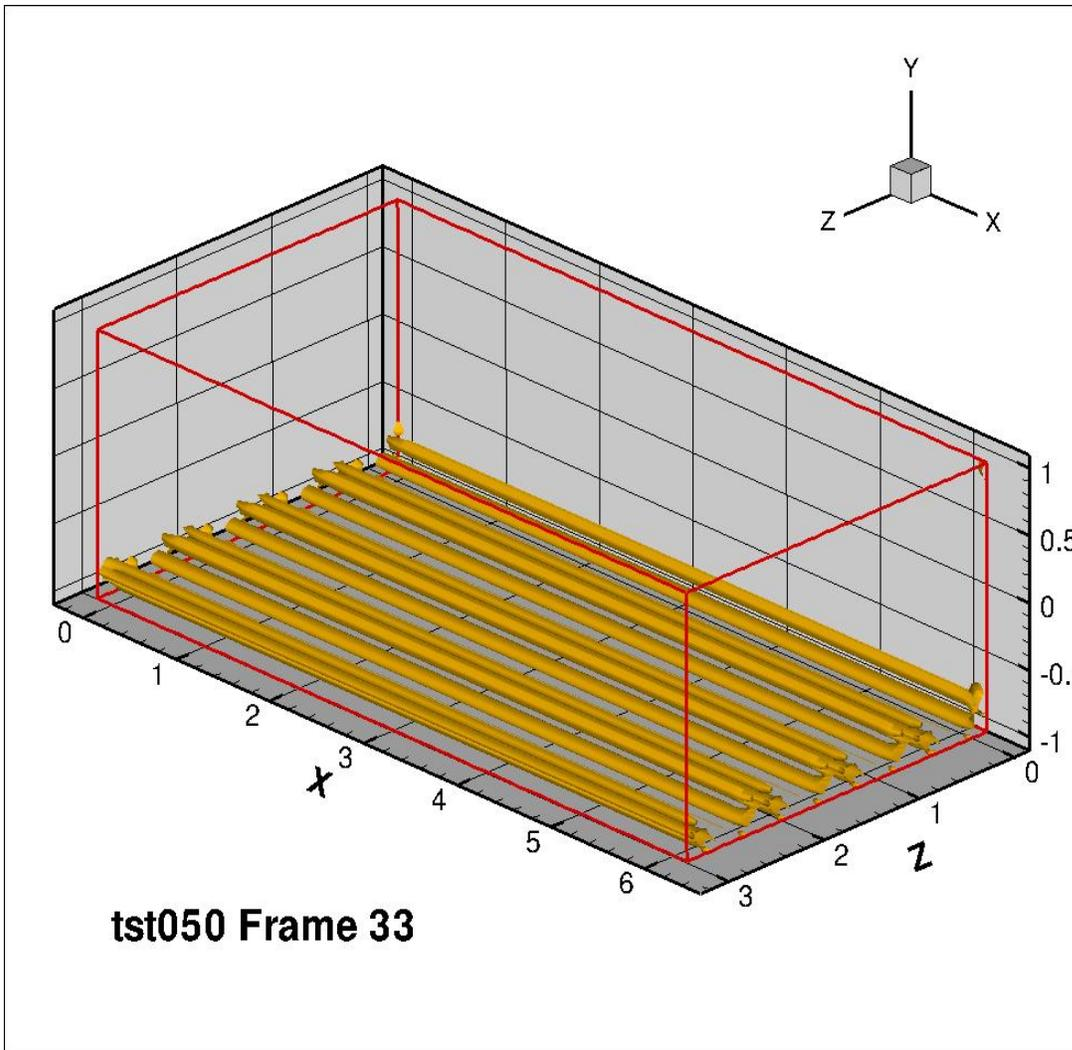
Figure 42: 8 counter rotating longitudinal vortices, frame 33
