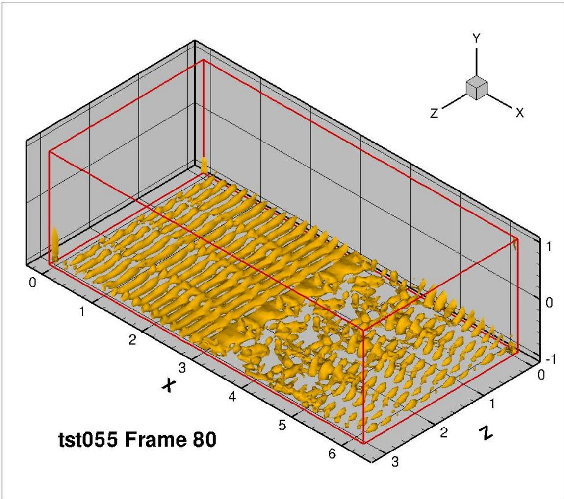
Figure 48: 12 longitudinal co-rotating vortices with trip bar, frame 80
