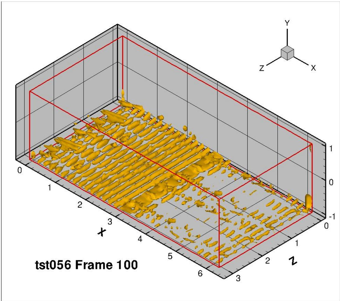
Figure 56: 12 longitudinal counter rotating vortices with trip bar, frame 100
