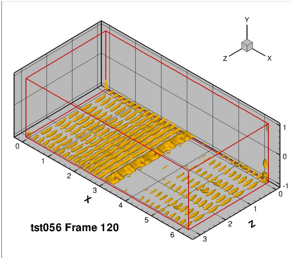
Figure 57: 12 longitudinal counter rotating vortices with trip bar, frame 120
