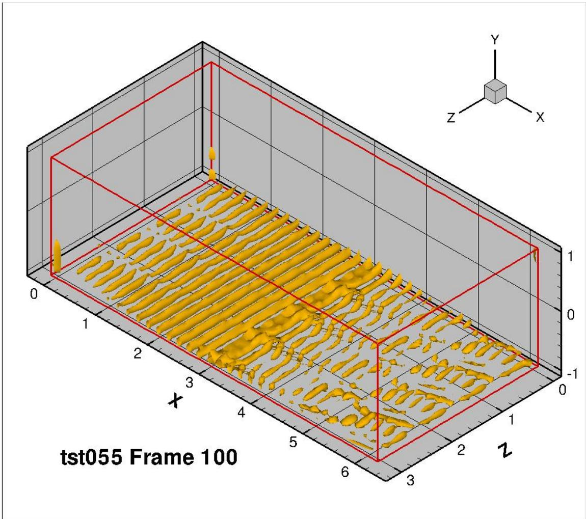
Figure 49: 12 longitudinal co-rotating vortices with trip bar, frame 100
