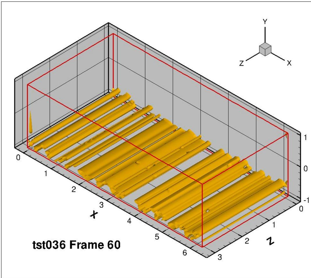
Figure 37: 8 lateral counter rotating vortices, frame 60
