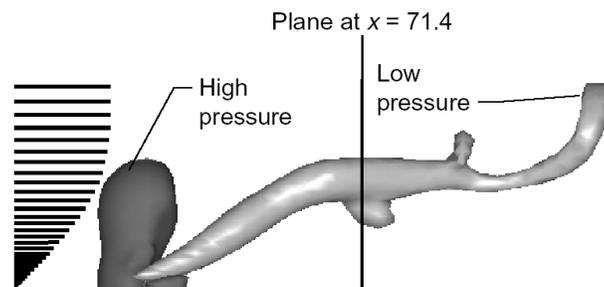
*Figure 16: Elevation view, hairpin vortex resulting from fluid injection,  $t=50.25$ , iso-pressure plot (Singer, Joslin, 1995)*
