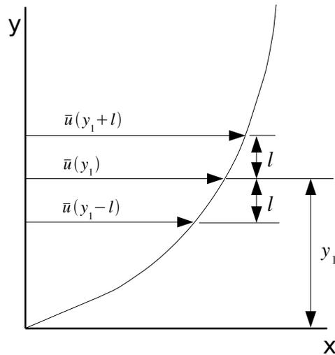
Figure 4: Diagram of Prandtl's mixing length theory
