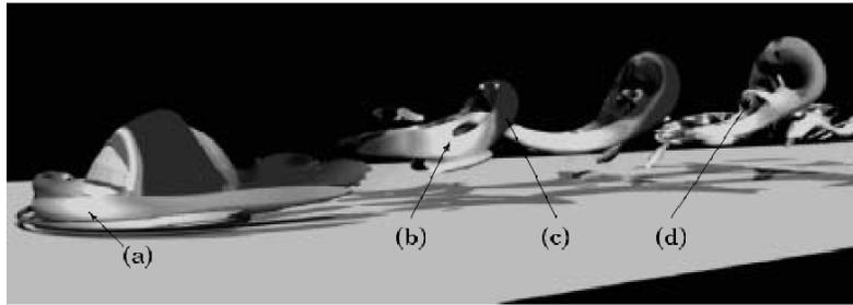
*Figure 20: Flow over hemispherical bump showing repeating hairpin vortices and upstream vortex at wall, (Tufo, Fischer, Papka and Szymanski, 1999)*
