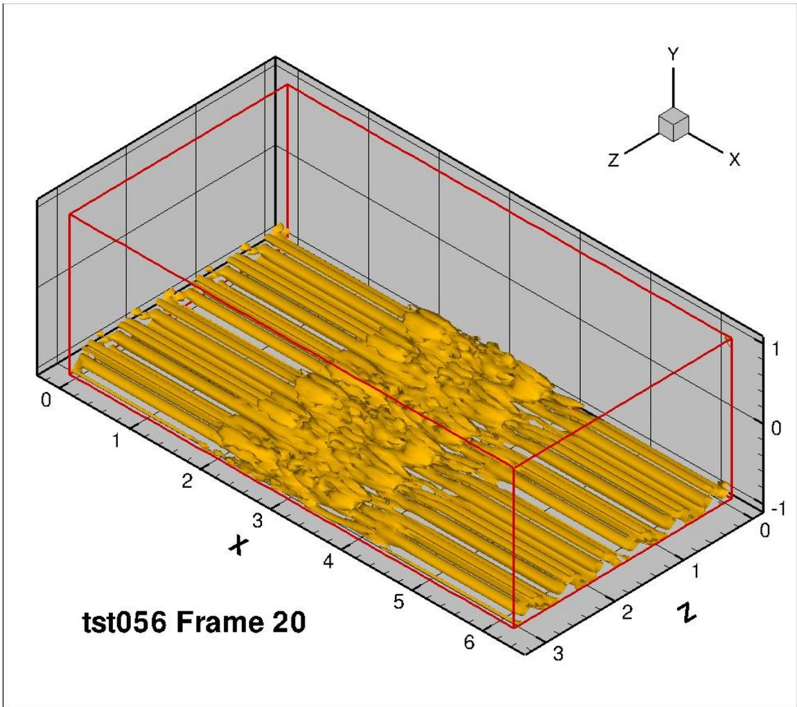
Figure 52: 12 longitudinal counter rotating vortices with trip bar, frame 20
