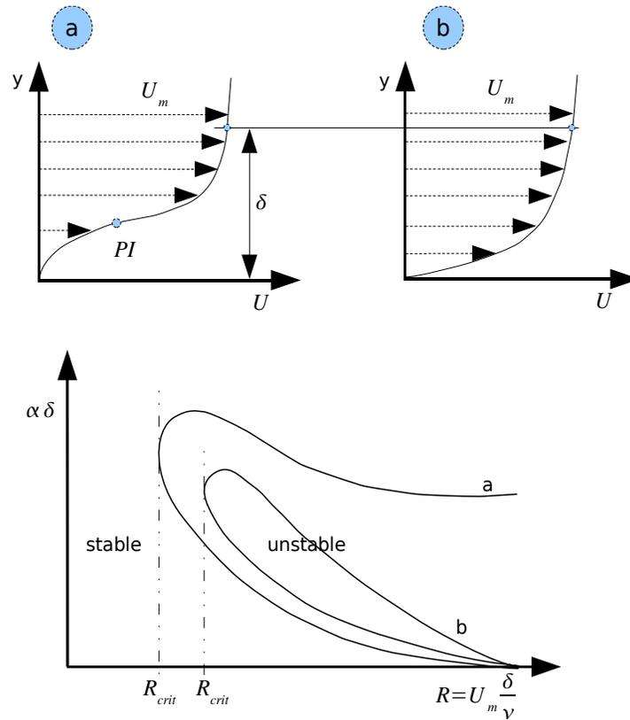
Figure 5: Boundary layer stability, a) boundary layer with inflection, b) boundary layer without inflection
