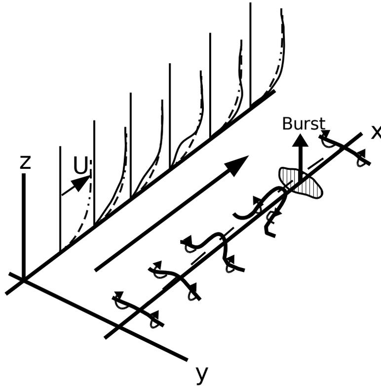
*Figure 8: Concept of turbulent burst cycle with hairpin vortex formation*
