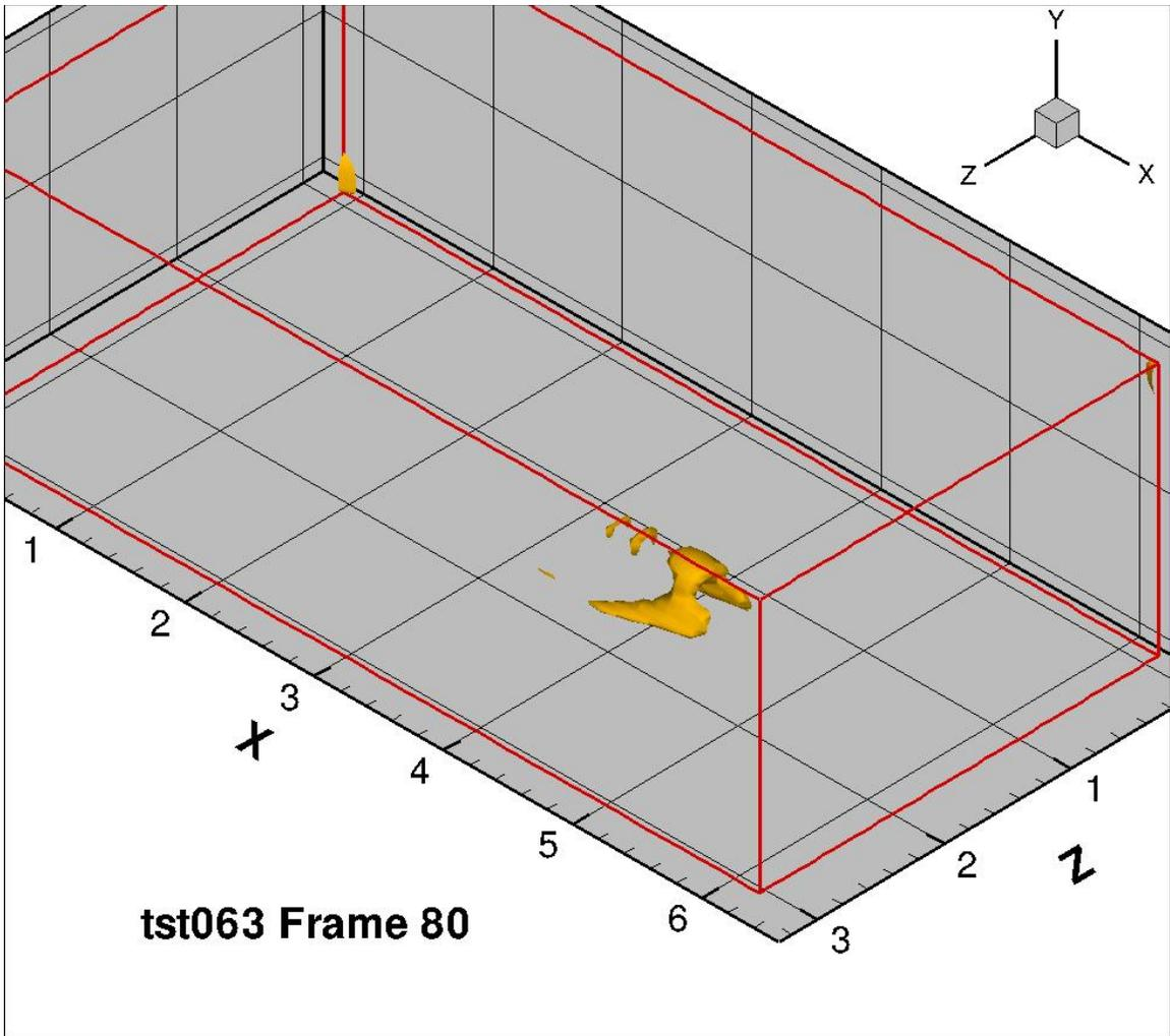
Figure 82: Vortices from fluid injection, frame 80
