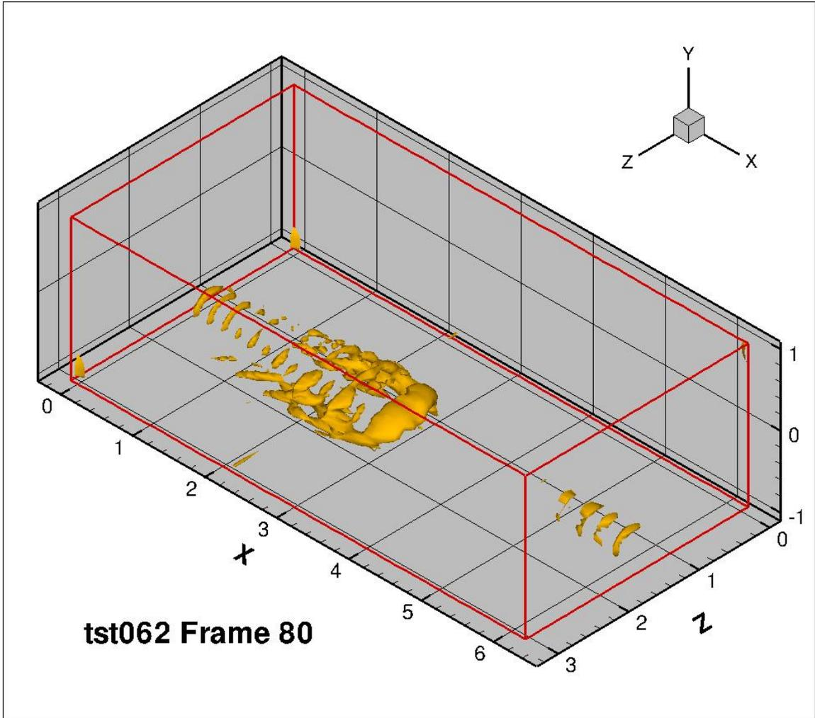
Figure 67: Rail and blade obstruction on channel wall, frame 80
