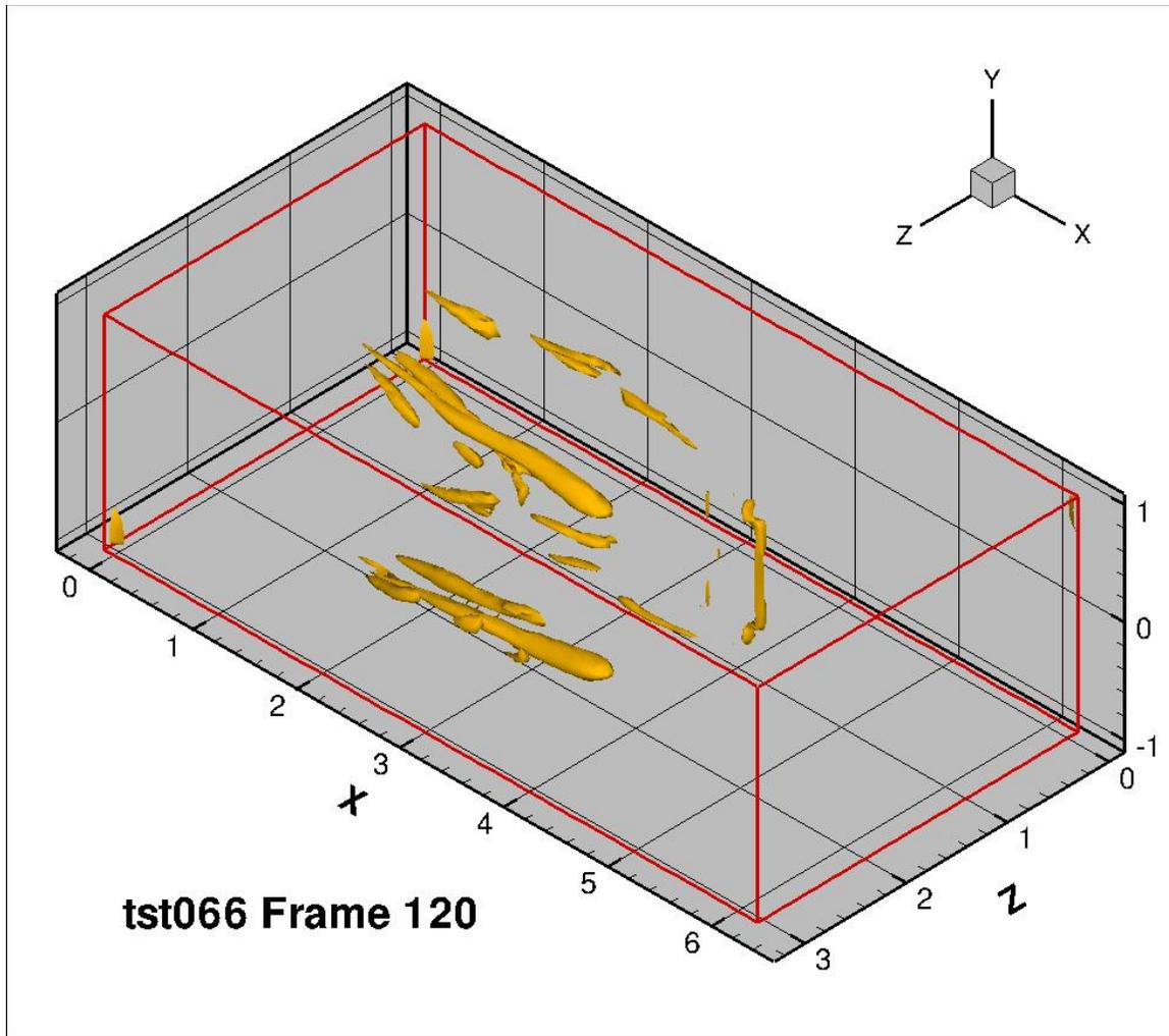
Figure 77: Narrow obstruction wall to wall, frame 120
