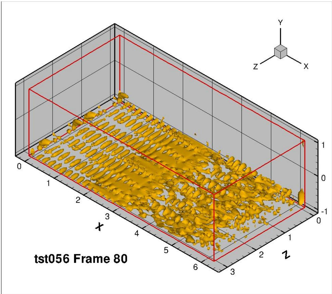
Figure 55: 12 longitudinal counter rotating vortices with trip bar, frame 80
