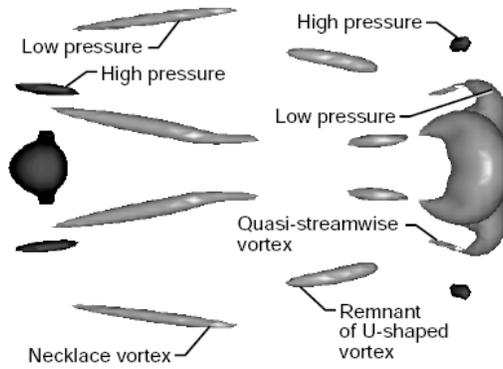
Figure 17: Plan view of turbulent structure,  $t=80.70$ , iso-pressure plot (Singer, Joslin, 1995)
