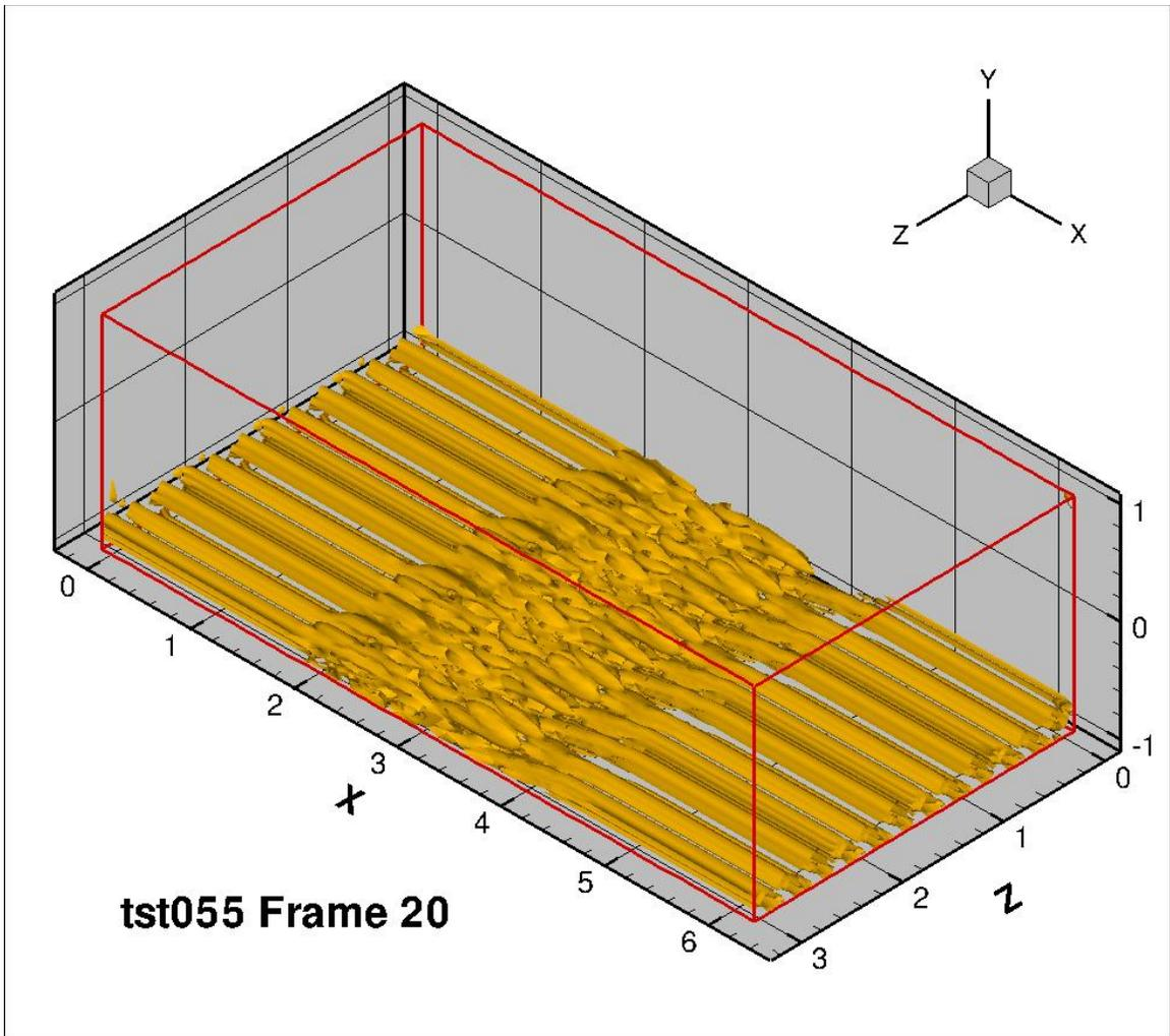
Figure 45: 12 longitudinal co-rotating vortices with trip bar, frame 20
