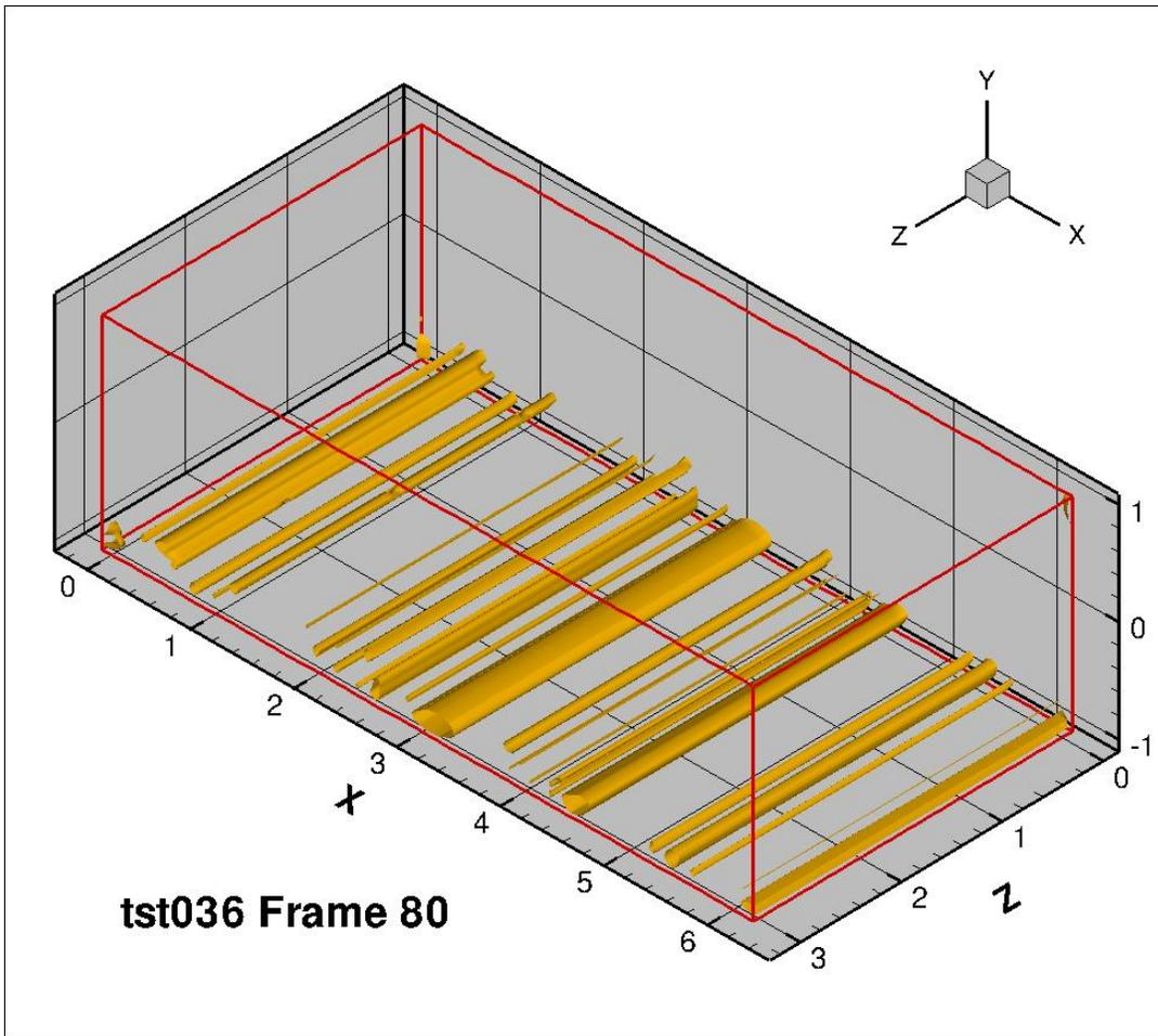
Figure 38: 8 lateral counter rotating vortices, frame 80
