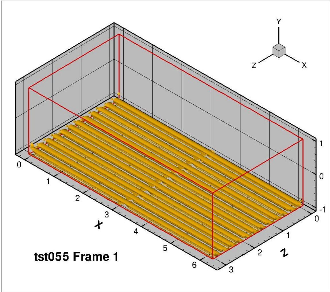
Figure 44: 12 longitudinal co-rotating vortices with trip bar, frame 1
