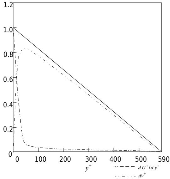
Figure 6: Decomposition of total stress in turbulent boundary layer, viscous stress, turbulent stress
