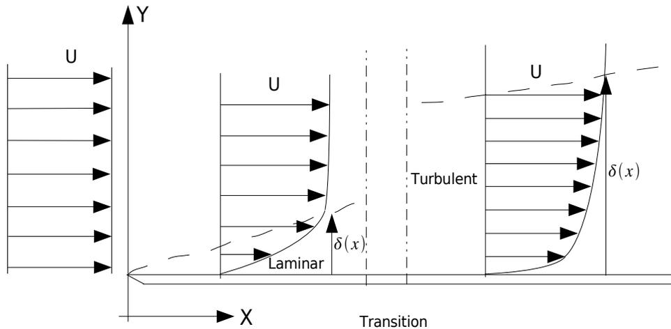
Figure 3: Transition to turbulent flow over flat plate
