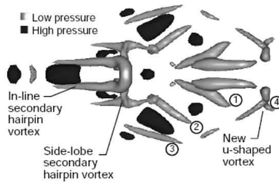
Figure 18: Plan view of turbulent structure,  $t=153.10$ , iso-pressure plot, (Singer, Joslin, 1995)
