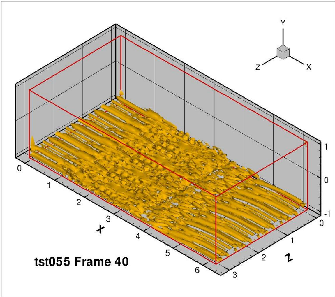
Figure 46: 12 longitudinal co-rotating vortices with trip bar, frame 40
