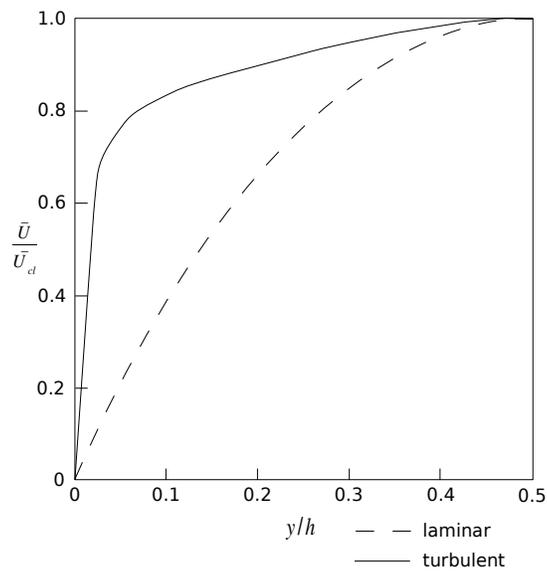
Figure 7: Boundary layer profiles, turbulent, laminar
