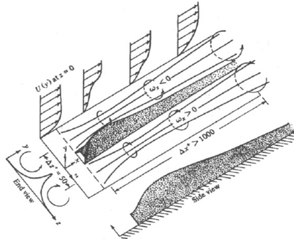
Figure 9: Counter-rotating streamwise vortices,
