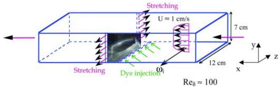
Figure 22: Diagram of experimental apparatus for vortex stretching, suction ports located opposed adjacent bottom wall, dye injected through bottom wall upstream of vortex. (Petitjeans, 2001)
