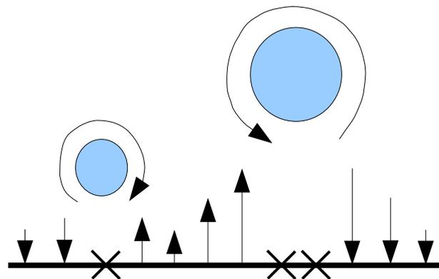
*Figure 85: Concept of suction and blowing to reduce angular momentum about vortical structures*
