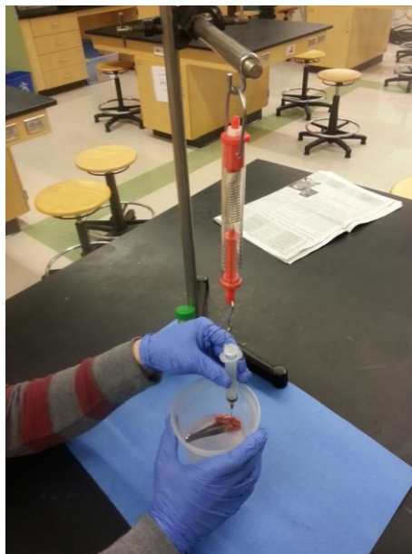
Figure 9: Force pullout test performed in rat liver
