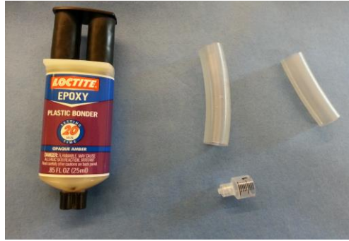
Figure 15: Luer lock attachment, Polyurethane tubing & plastic epoxy
