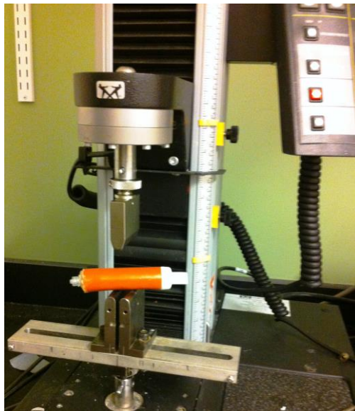
Figure 49: Compression of prototype with Instron Machine
