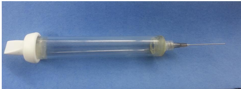
Figure 50: PVC tubing with Duckbill Valve & Luer Lock attachment to a 22-Gauge Needle
