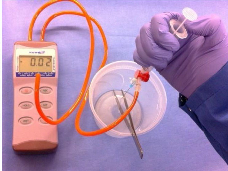
Figure 10: FNA procedure using a three-way valve
