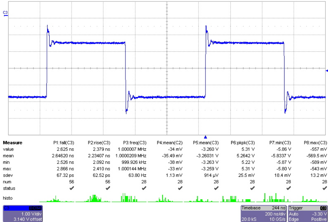
Figure 46: 1m Cable, PCB Output, Terminated, 1MHz Square Wave Input
