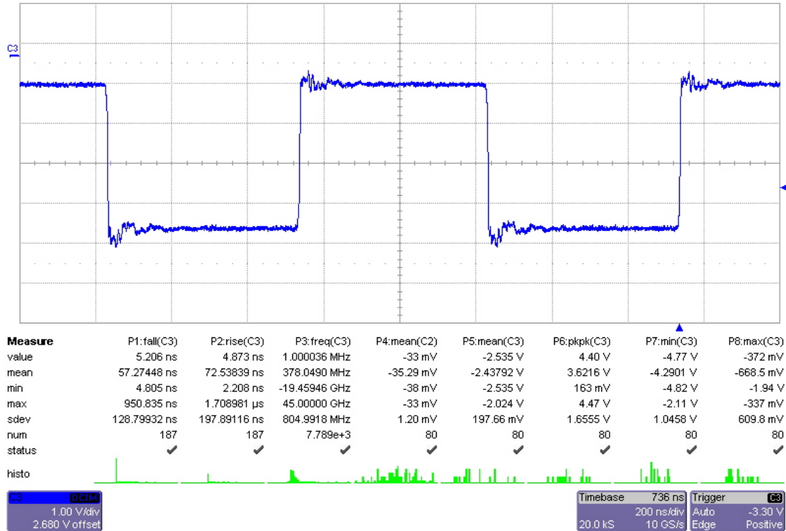
Figure 42: 3m Cable, SWD-119 Output, Terminated, 1MHz Square Wave Input
