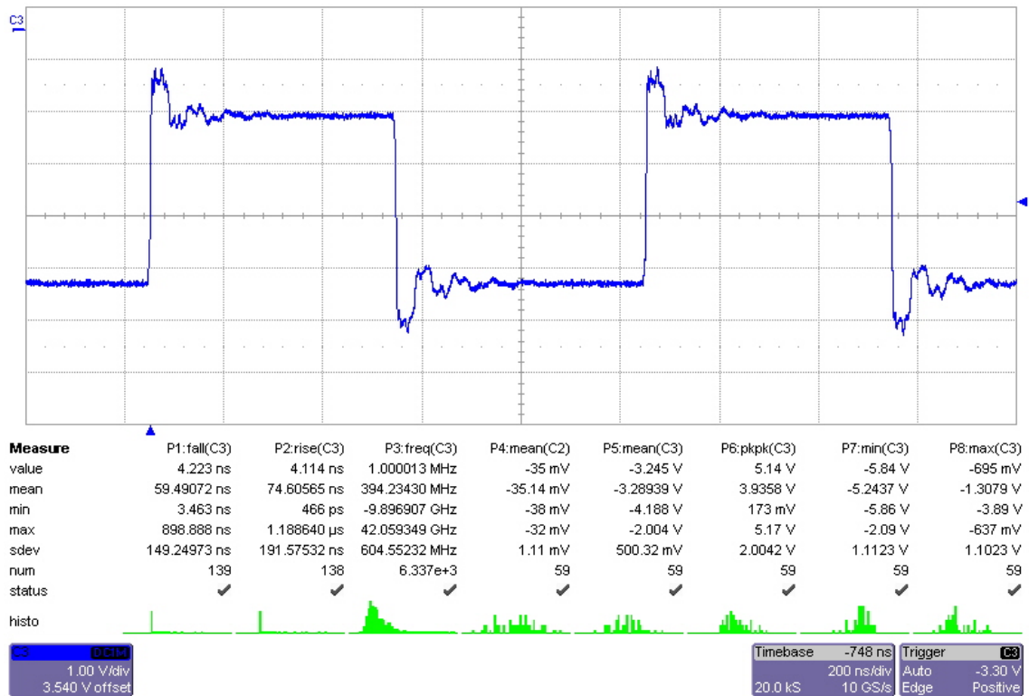
Figure 41: 3m Cable, PCB Output, Terminated, 1MHz Square Wave Input
