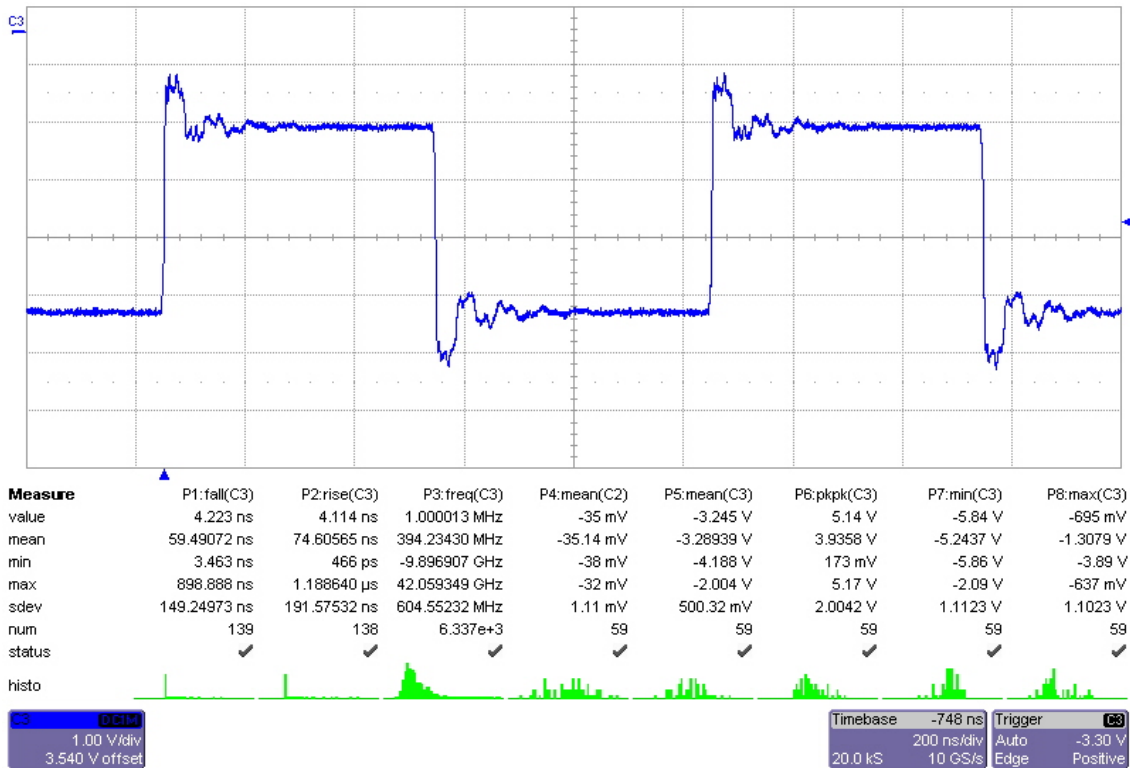
Figure 88: 3m Cable, PCB Output, Terminated, 1MHz Square Wave Input
