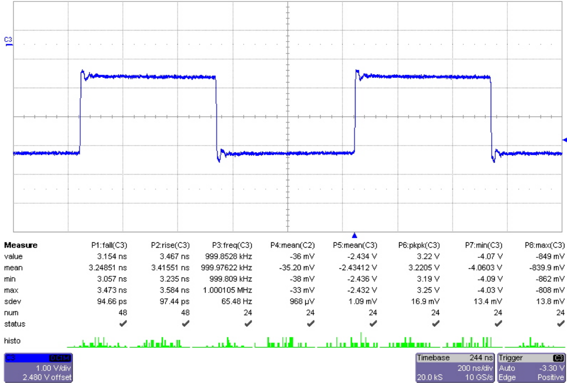
Figure 93: 1m Cable, SWD_119 Output, Dual Termination, 1MHz Square Wave Input
