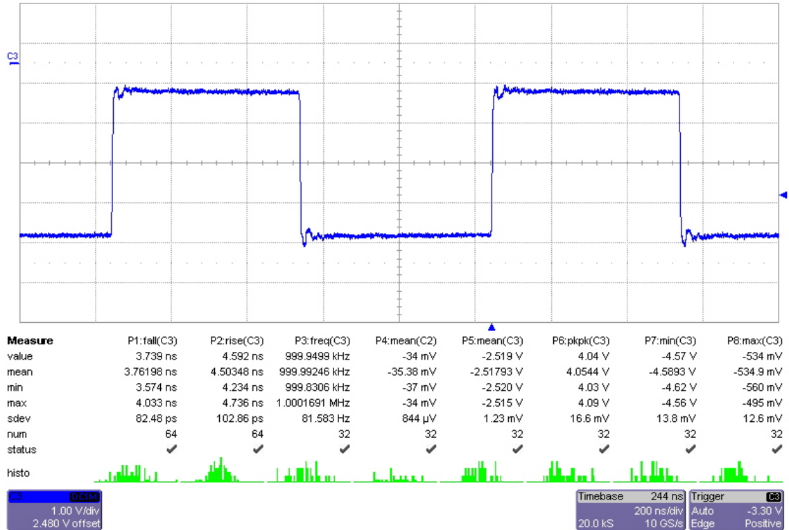
Figure 85: 1m Cable, SWD-119 Output, Terminated, 1MHz Square Wave Input
