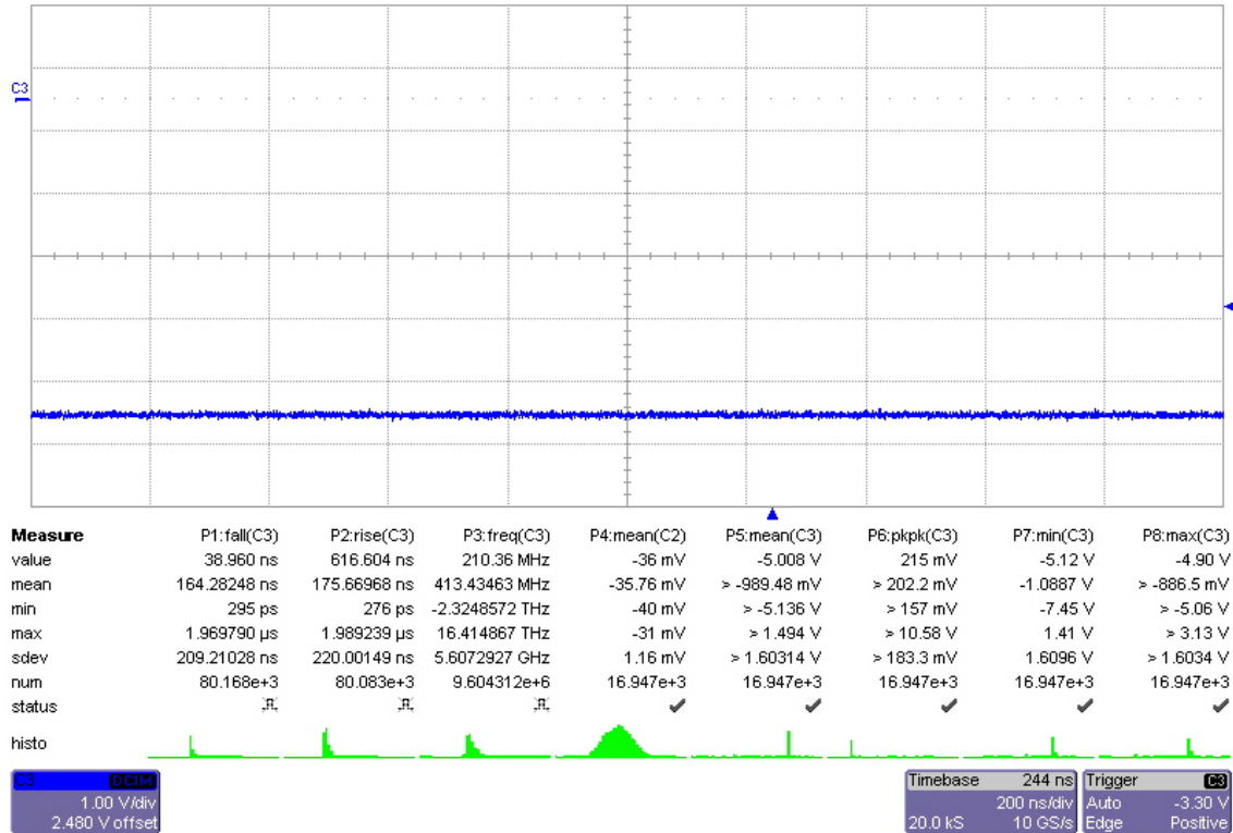
Figure 40: No Cable, SWD-119 Output, No Termination, Static 5V Input
