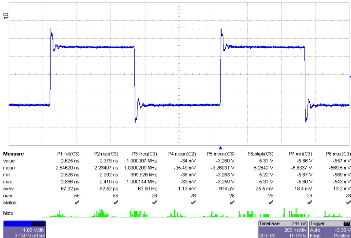
Figure 84: 1m Cable, PCB Output, Terminated, 1MHz Square Wave Input
