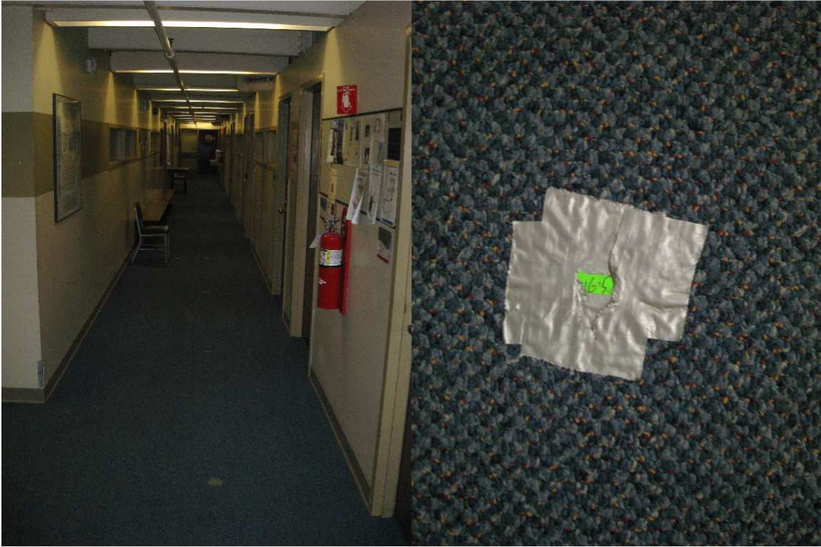
Figure 6.1: The position markers outlining the locations of ZUPTs along the length of the test course.
