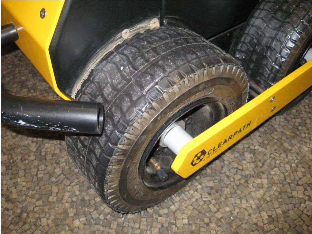
Figure 6.3: The wheels of the Husky A100 UGV coated in duct tape to reduce the coefficient of friction between the wheels and the carpeted floor.
