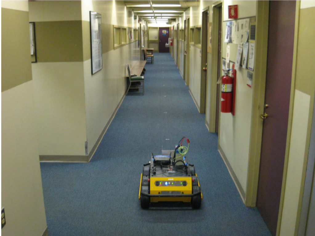
Figure 6.5: The Husky A100 UGV positioned at the beginning of the test course.
