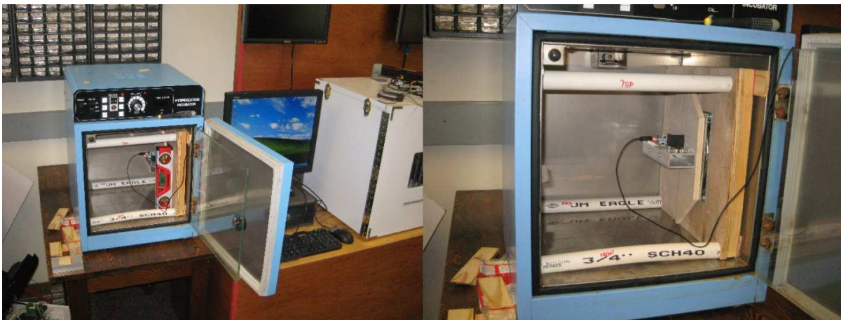
Figure 4.18: The Multi-Angle Experiment test fixture enclosed in the hybridization incubator. The PVC pipes are used to ensure that the test fixture remains stationary and level during the course of the experiment.
