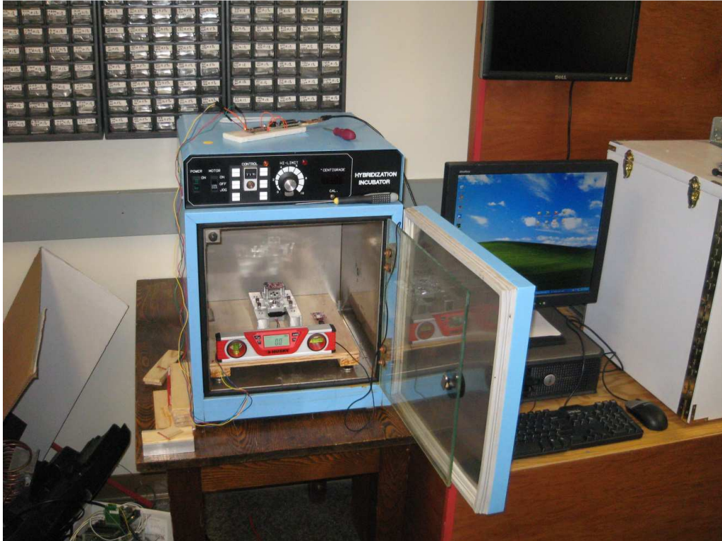
Figure 4.21: The Rate Table Experiment test fixture enclosed in the hybridization incubator.
