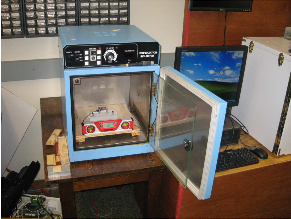
Figure 4.16: The test fixture for the Power Cycle Experiment enclosed in a hybridization incubator.
