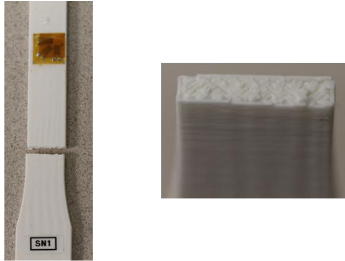
Figure 2-24 45/-45 Z-axis Oriented Test Article after destructive Tensile Testing (Left) Fracture Pattern (Right)
