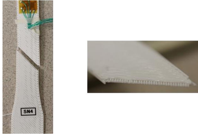
Figure 2-32 45/-45 n = 1 Test Article after destructive Tensile Testing (Left) Fracture Pattern (Right)
