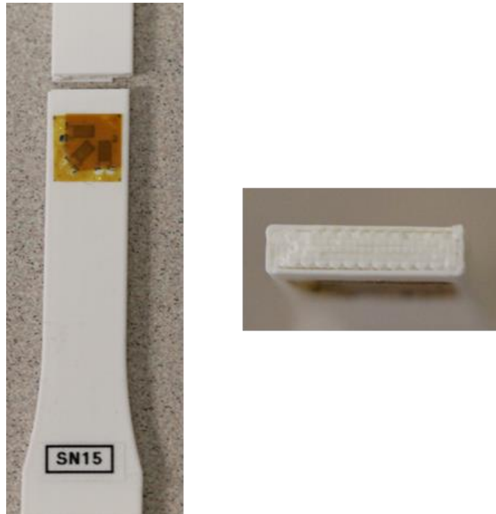
Figure 2-27 0/90 Z-Axis Oriented Test Article after destructive Tensile Testing (Left) Fracture Pattern (Right)
