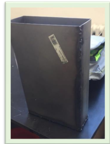
Figure 3: Metal box created to make mold of 3D flipper in.
