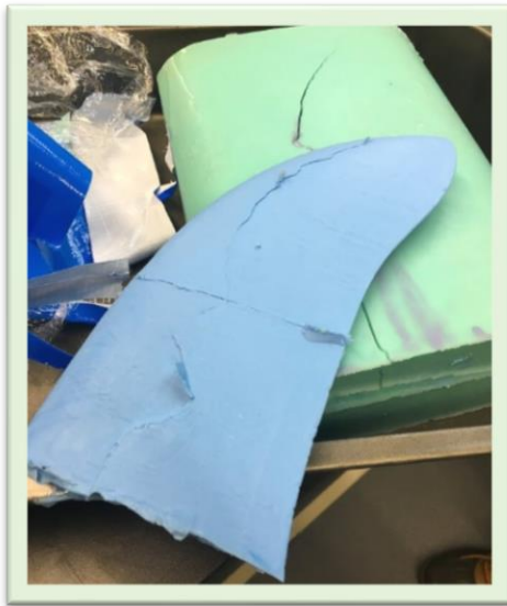
Figure 8: Final prosthetic flipper removed from mold.
