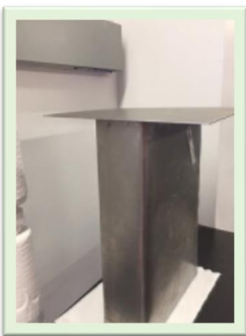
Figure 6 (Right): How the flipper should look once the mold hardens. Approximately 1/2 inch should be showing.
