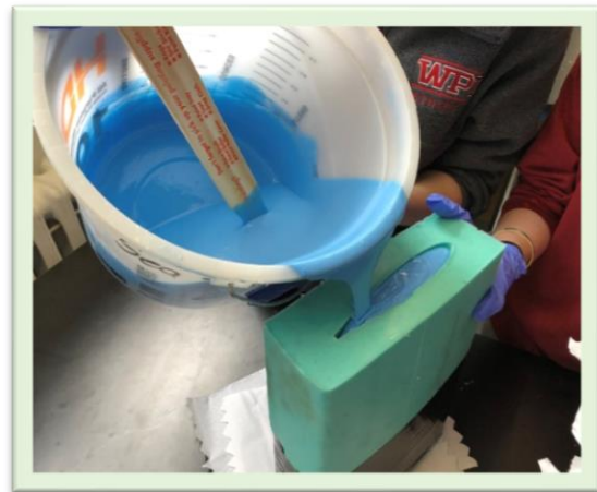
Figure 7: Pouring the Smooth-Sil 950 into the mold
