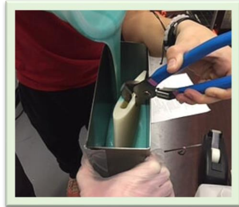
Figure 4: Holding the 3D printed flipper in place while the mold mixture is poured around the flipper.
