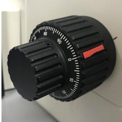
Figure 26: Z-Axis Coarse and Fine Focusing Dials of Leica Light Microscope
