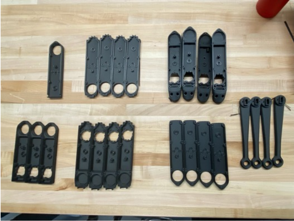
Figure 12: Actuator Module Shells printed in Onyx
