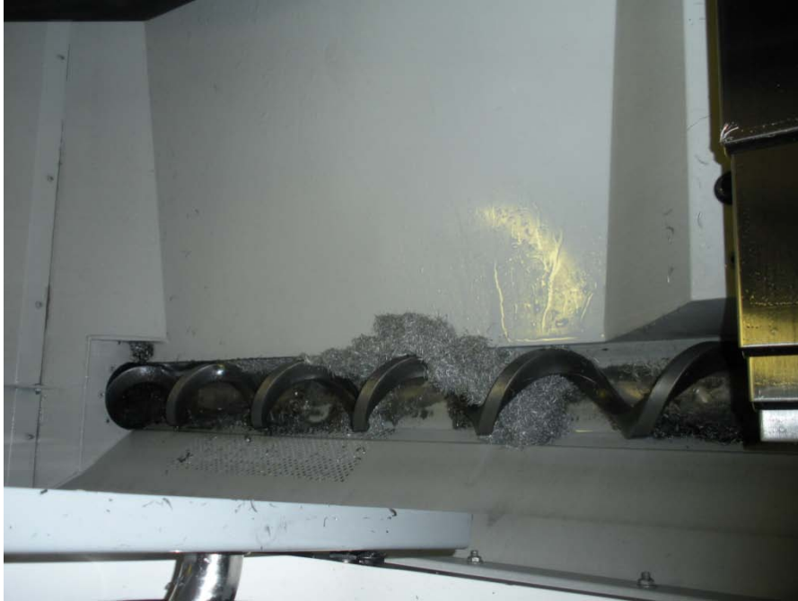
Figure 9: Recycling mechanism in Haas VF-4SS
