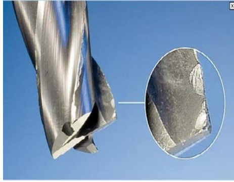
Figure 13: Tool wear on end mill
