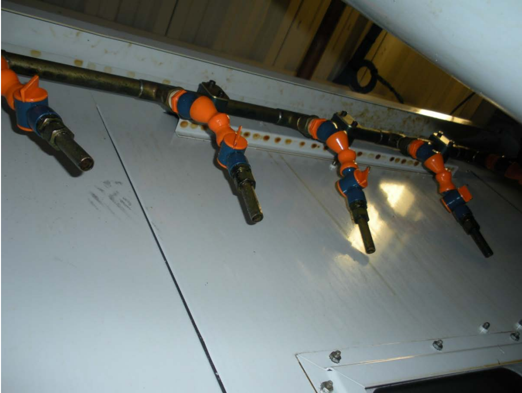
Figure 7: Installment of the nozzles in Haas Mill Drill Center
