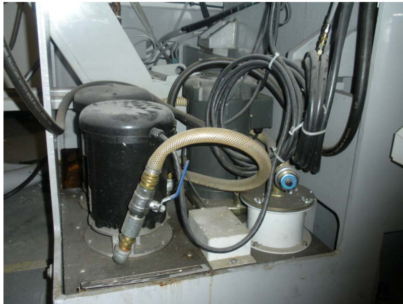
Figure 4: Coolant pump for Haas Mill Drill Center
