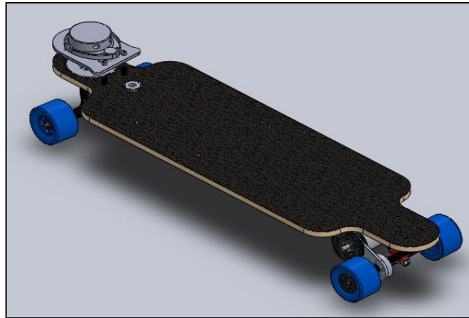
Figure 9: Preliminary Board SOLIDWORKS Design
