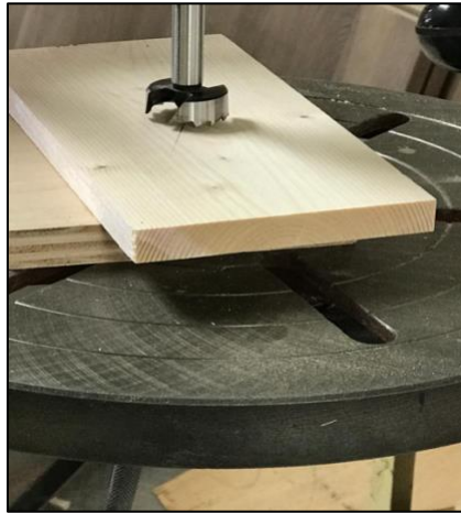
Figure 16: Boring hole in side of vacuum forming machine
