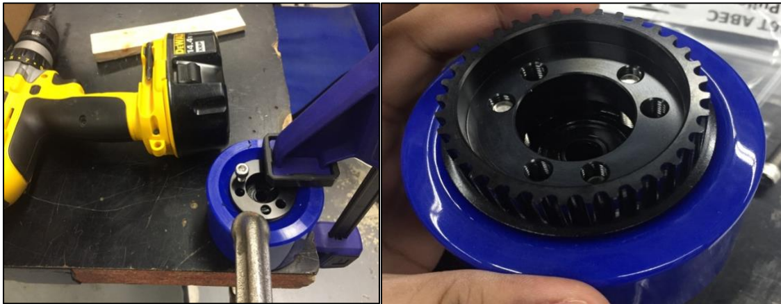
Figure 24: Wheel clamped for drilling bolt holes.
