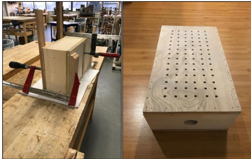
Figure 18: a) Left: Construction of vacuum forming machine and b) Right: Final
