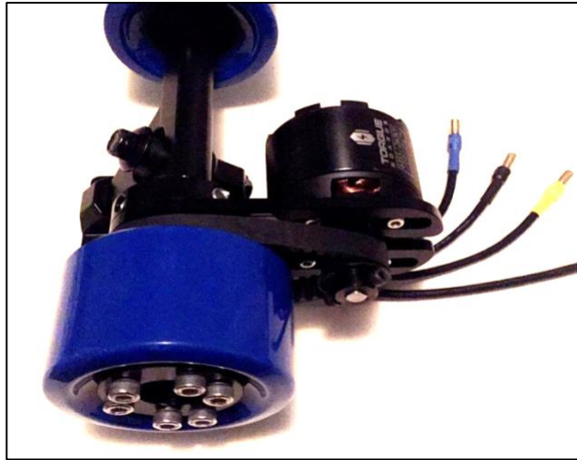
Figure 25: Assembled drivetrain on rear truck
