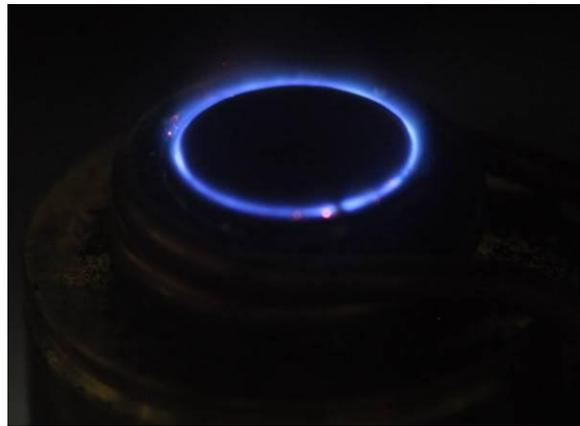
**Figure 3.7: Image of premixed methane-oxygen pilot flame**
